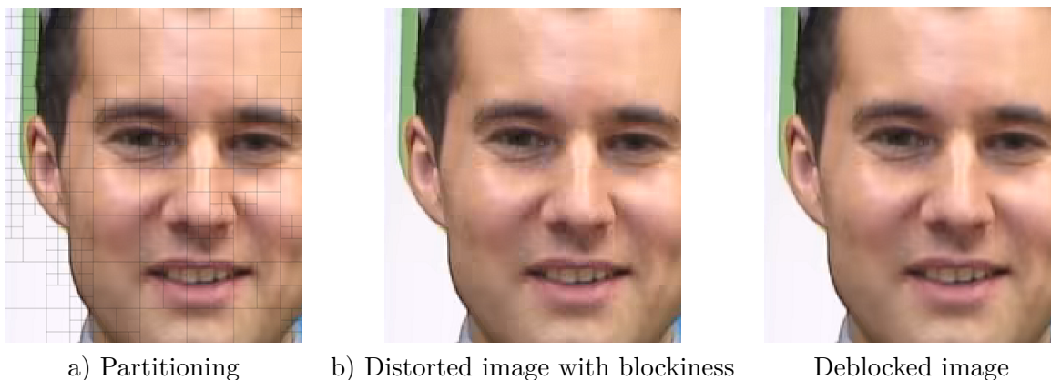
Figure 1.9 – Impact of partitioning on block artefacts and the DBF as its efficient solution.
