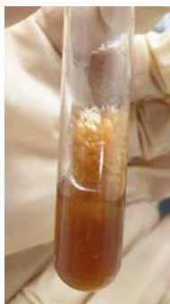
Figure S68 – Content of the glass tube at the end of the reaction, in the optimized conditions. Because of its low solubility in toluene, succinic anhydride precipitated.
