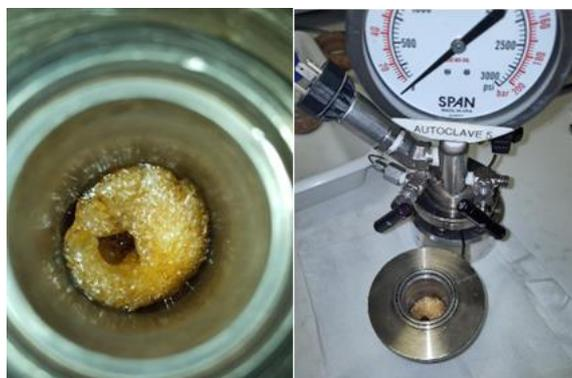
Figure S69 – Content of the large-volume autoclave at the end of the reaction, in the optimized conditions. Because of its low solubility in toluene, succinic anhydride precipitated.
