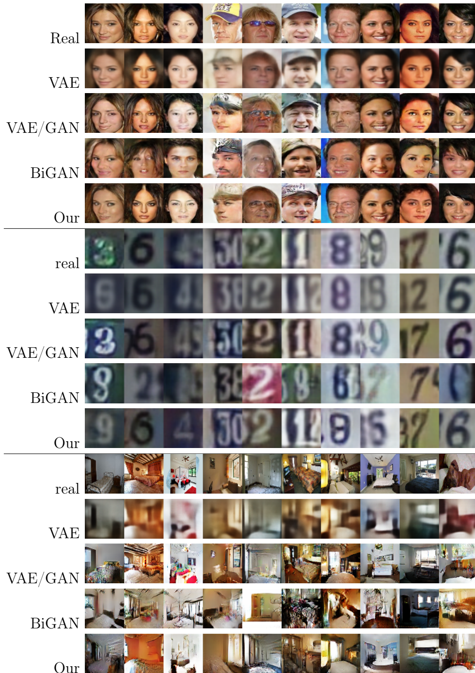
Figure 3.8: Qualitative comparison of the quality of reconstructions between several frameworks namely VAE, VAE/GAN, BiGAN and our model on three datasets: CelebA, SVHN and LSUN bedroom.
