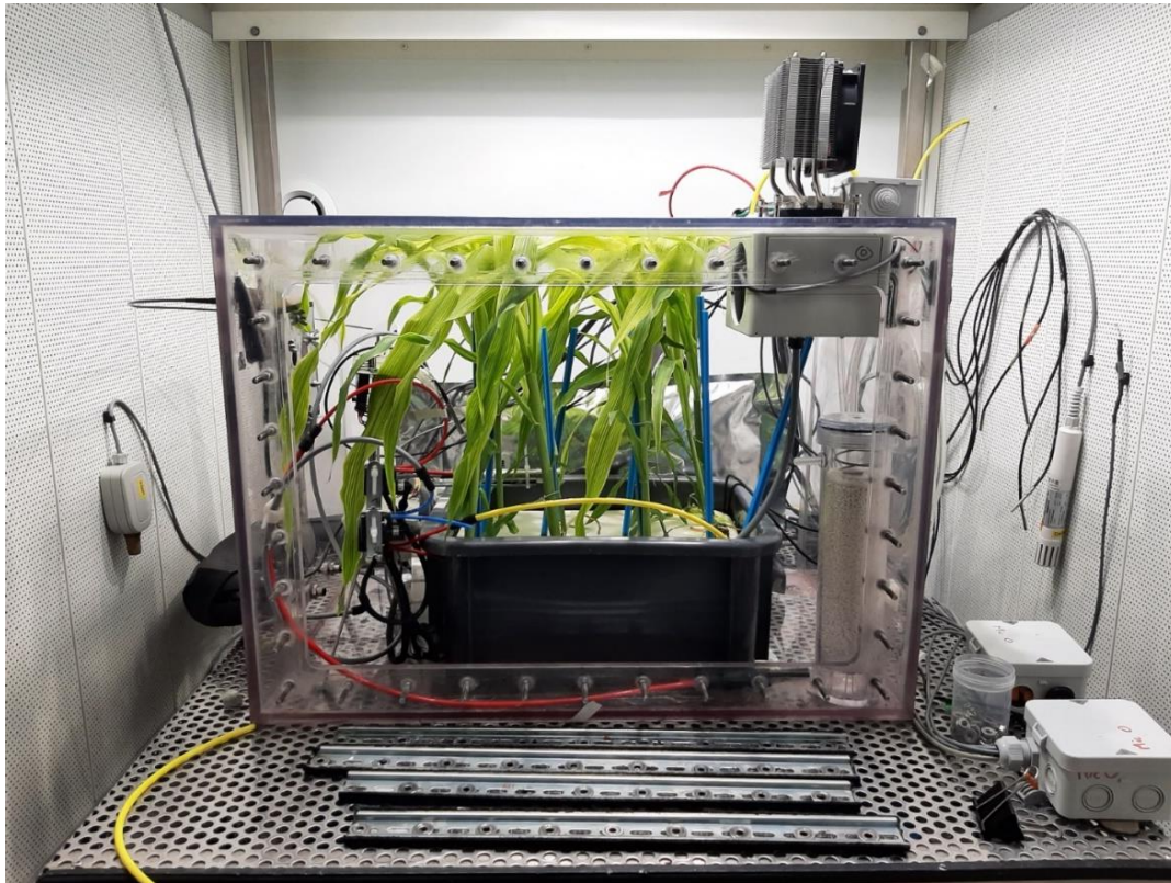
Figure 1. The set-up of the closed chamber system hosting a vegetation-soil atmosphere analogue of the terrestrial biosphere. (a) Schematic of the closed chamber setup used for the terrestrial biosphere model. The closed chamber was enclosed in a larger growth chamber. Main environmental parameters inside the closed chamber were actively controlled and monitored: temperature ( T ), light intensity, \text{CO}_2 , relative humidity ( \text{RH} ), pressure differential ( \Delta P ). The water cycle in the closed chamber is shown in blue. (b) Photograph of the closed chamber used in the experiment with Zea Mays .
