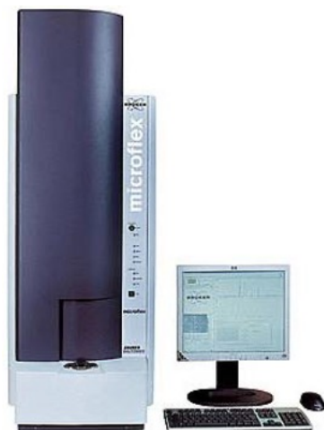
FIGURE 2.1 – Appareil MALDI-TOF Source : A. Godmer
