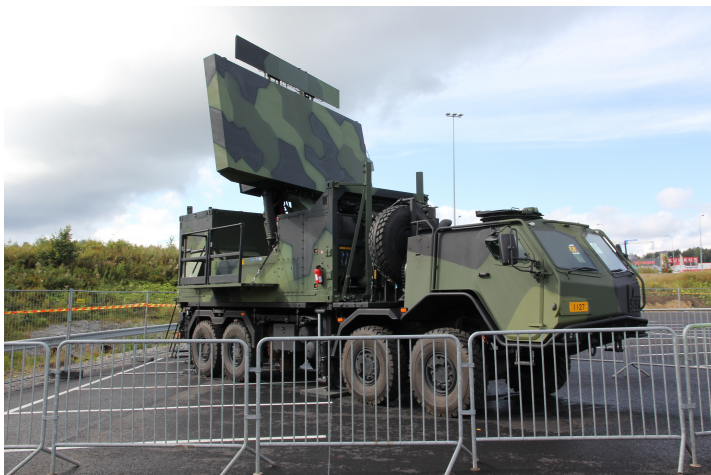
(a) GM400 "Ground Master" S-Band Radar phased array radar, source: Wikimedia.org
