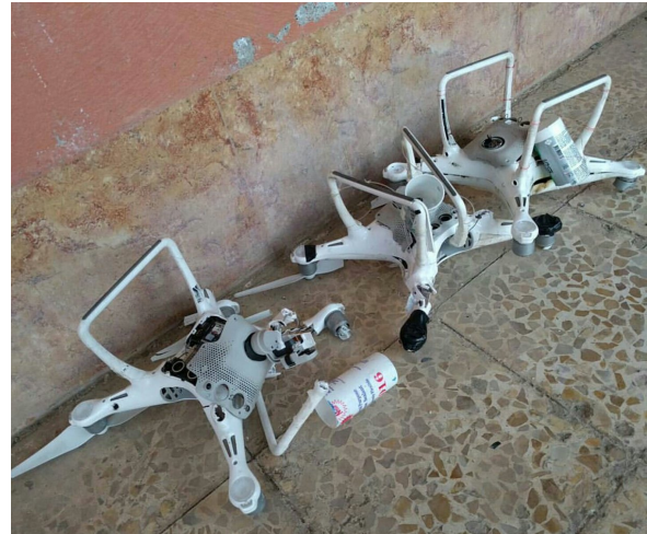
(b) DJI Phantom used as improvised weapon carrier by the Islamic State in Iraq and the Levant, source: Waters 2017
