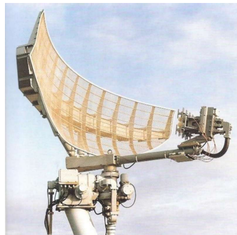
(b) DRBV 15A "Sea Tiger" S-Band Radar radar with focusing parabola, source: radar-tutorial.eu
