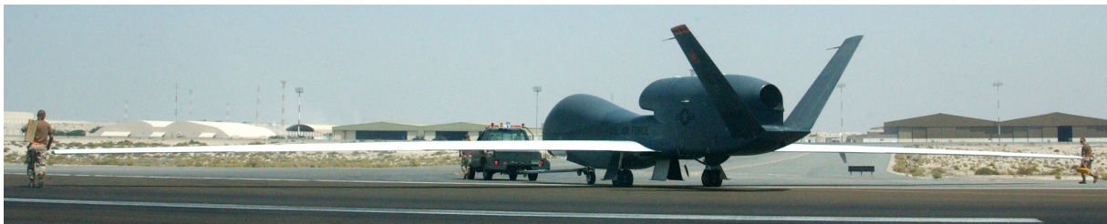
(c) RQ-4 Global Hawk High Altitude Long Endurance (HALE) UAV, source: Wikimedia.org
