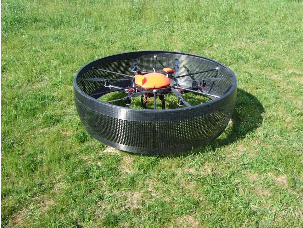
Figure 4.14: Picture of the UAV used in the measurement campaign. The crown carbon fiber crown was not fitted on the UAV during the campaign.
