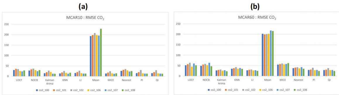
Figure 2.17 – Comparison of the RMSE for some CO 2 sensors of room 219 using the MCAR missing data generation mechanism and for 10 % (a) and 60 % (b) of missing data. From (Es-Sabar 2022).
