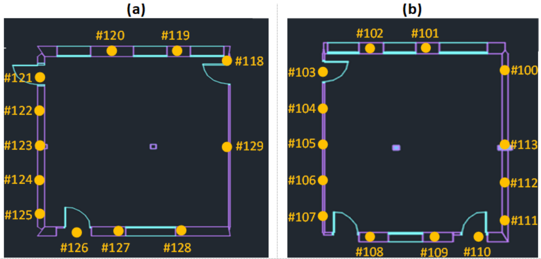
Figure 2.10 – Multiphysical sensor locations in room 114 (a) and 219 (b).
