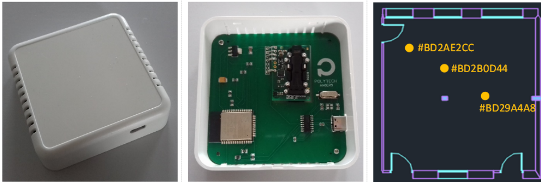
Figure 2.11 – Multiphysical sensor board at student’s locations in the classroom 219.
