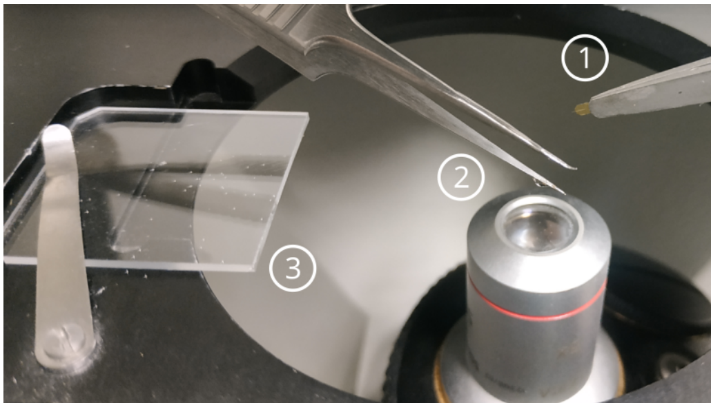
Figure 9.3: The setup used for microfabrication of our probes. Two micro-manipulator are used to move tweezers holding the cantilever (1) and glue (2). Polystyrene beads are deposited on a microscope slide (3).
