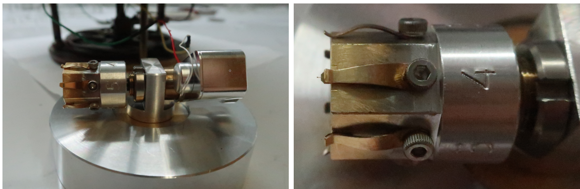
Figure 9.6: Left: The cantilever holder. The left part is a hexagonal head and can hold 6 cantilevers. The right part is vacuum proof piezo inertial motor that can rotate the head. Right: Close-up on the head. 6 cantilevers chips are held so that the cantilevers themselves can be coated without shadow.
