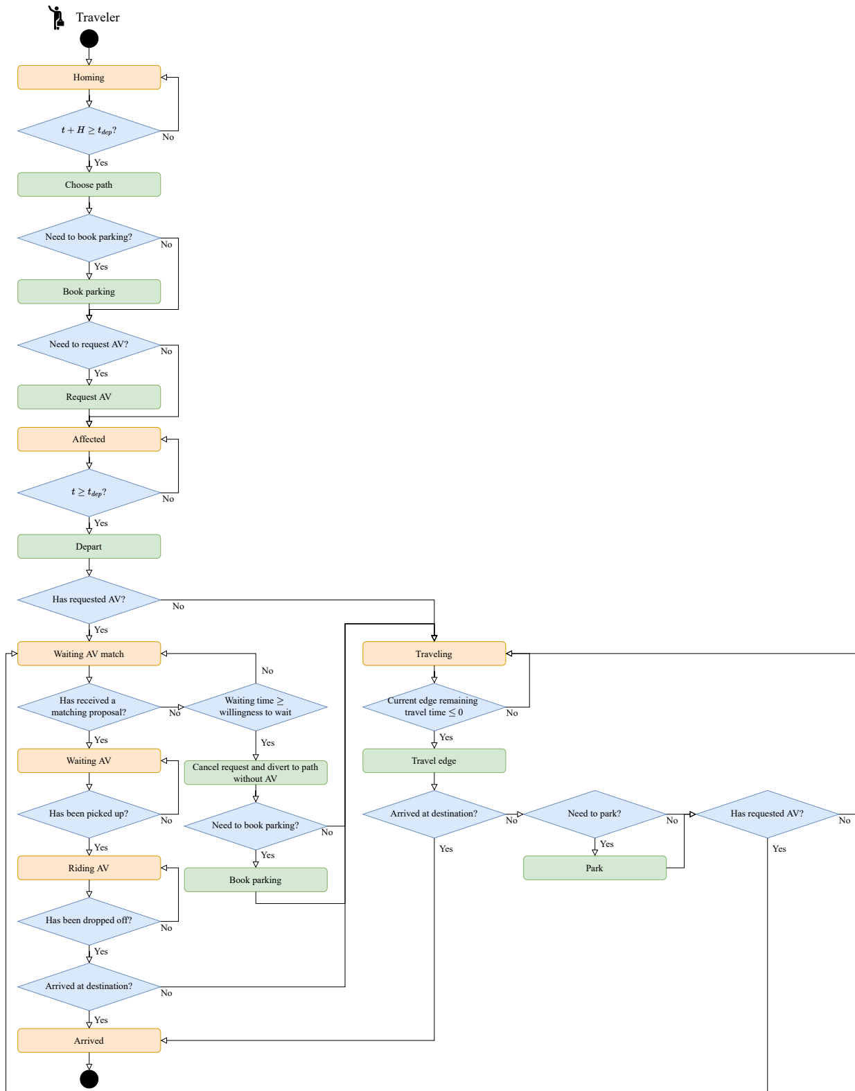
FIGURE B.1 – Flow chart of traveler agent in the agent-based simulation platform used for chapter 4.
