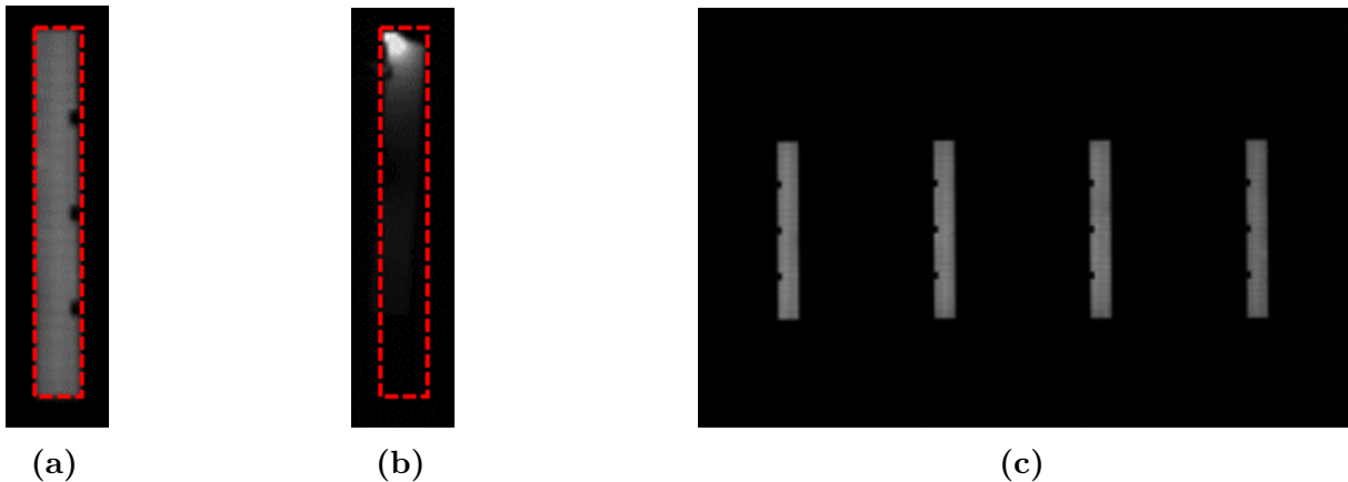
Figure 3.20: Electroluminescence response of a single III-V/Si solar cell ( 1.5 \times 13 \text{ mm}^3 , see red-dashed-line) with: (a) homogeneous radiative emission indicating the absence of fractures (red dotted box represents the cell surface); (b) with a point peak of luminosity on the cell, and the rest shaded, indicating the existence of defects in the semiconductor structure. (c) EL of an interconnected string after wire-bonding.
