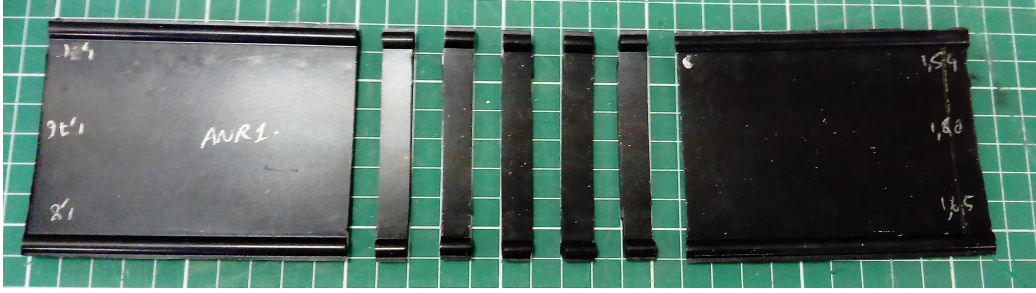
Figure 2.4: Samples extracted from the large plate: two large 100 \times 65 \text{ mm}^2 samples and five 10 \times 65 \text{ mm}^2 samples for traction tests. The plate displayed is ANR1. The dimensions of the white squares in the background are 1 \text{ cm}^2 .
