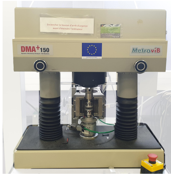
Figure 2.9: DMA testing setup. On the left stands the MetraViB DMA+150 machine, a dynamic testing machine with 150 N stiffness.
