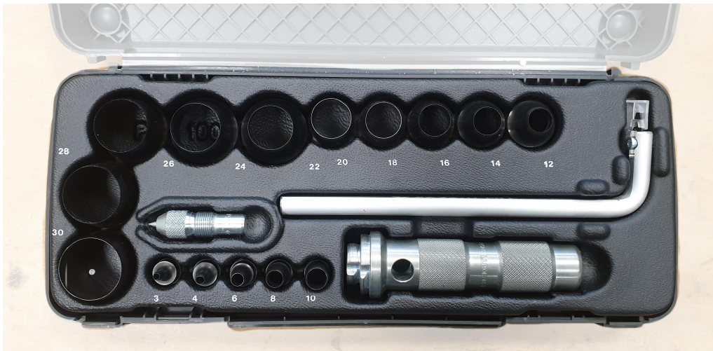
Figure 7.1: Hole punchers available for sample design. The diameters vary from 3 to 30 mm.
