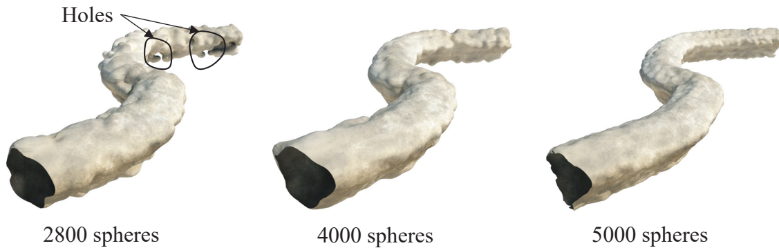
FIGURE 7.20: Tunnels generated with different amount of spheres. Using a small amount of spheres is more compact in memory but can lead to unwanted bumps and defects in the approximation of the tunnel.
