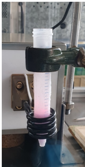
Figure 22: Photo of the setup for the inductive thawing of the fibroblast-containing 3D tissue models. Special acknowledgements to Anika Hoeppel for the figure preparation.
