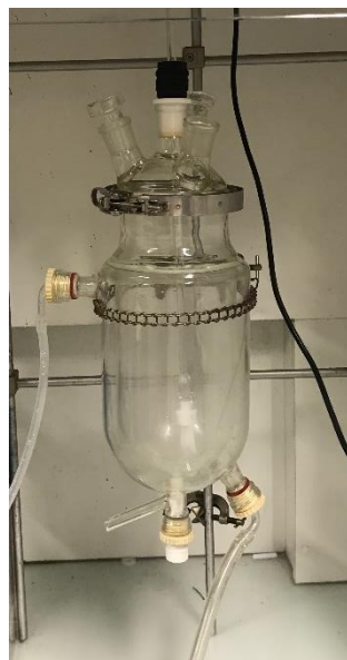
Figure A.17 - The used reactor with thermal shell
