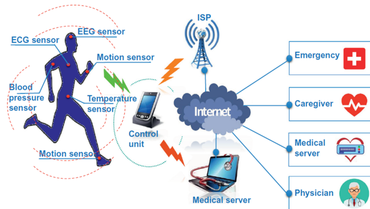
FIGURE 2.7: Framework for intelligent health care monitoring systems (HCMS) [Subasi et al., 2020].
