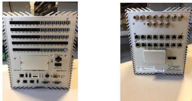
Figure 4.7. Customized Speedgoat real-time target machine
