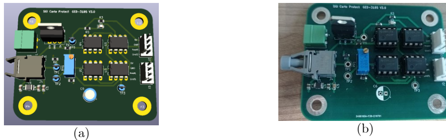
Figure 4.34. Protection board (a) concept, (b) final board
