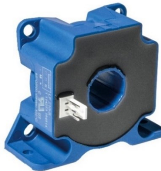
Figure 4.22. LEM LF 210-S for load current measurement
