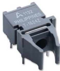
Figure 4.26. AFBR-1624Z fiber optic transmitter
