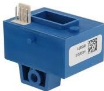
Figure 4.33. LEM transducer HASS 50-S
