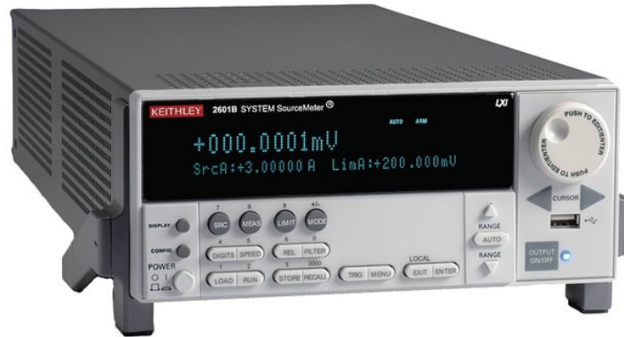
Figure 4.48. Source Meter Unit Keithley 2612B
