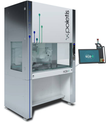
Figure 9.2.: Poietis NGB device. NGB integrates (i) computer-assited design (CAD software), (ii) automated robotic bioprinting with laser-assisted technology, (iii) multimodal extrusion and micro-valve heads to print the biomaterial, and (iv) motinoring of the tissue maturation via cell microscopy and image processing tools. More details in Section 9.3.
