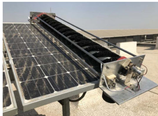
Fig. 11. Water-free service unit (Deb and Brahmabhatt, 2018).
