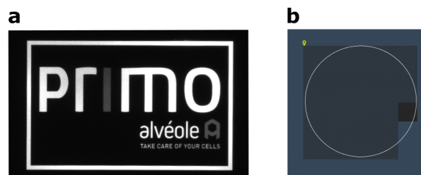
Figure A.2: Micropattern preparation with Leonardo software. a , Photograph of the calibration image obtained using a 10x objective and a coverslip with a yellow highlighter. The letters appear with sharp edges and different intensities. b , Photograph of a scan using the circle tool to obtain a bright-field image of your well.
