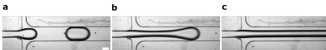
Figure 3.12: Flow regimes in a flow-focusing channel. a , Dripping regime. b , Jetting regime. c , Threading regime. Scale bar = 100 \mu\text{m} .
