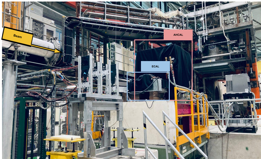
FIGURE 4.19: Picture of the detector set up and beam pipe. ECAL is placed in front of the AHCAL prototype.
