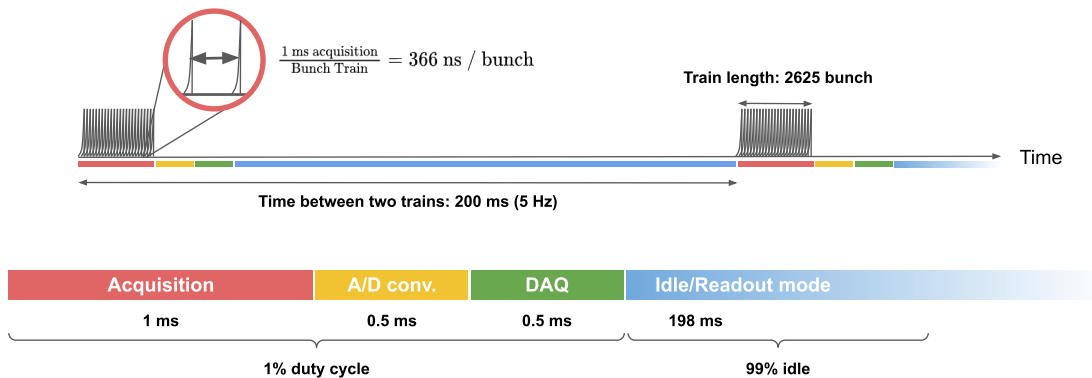
FIGURE 4.15: Bunch structure of the ILC electron and positron beams.
