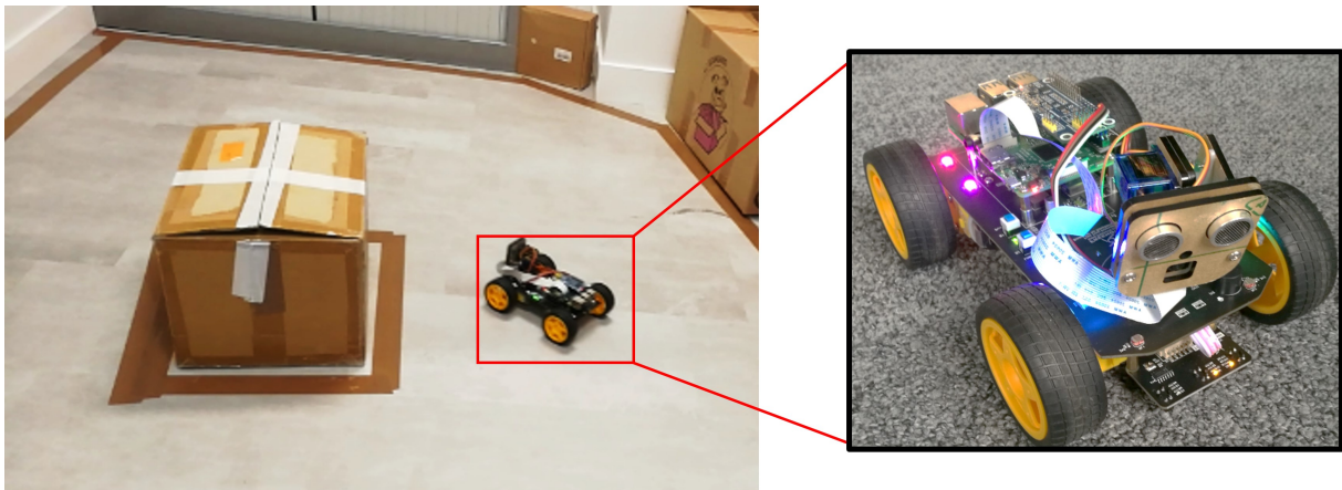
Figure 5.2: (left) Arena for the SCR to traverse for data collection and attack testing on the presented IDS (right) The SCR with on board Raspberry Pi and various sensors and network communication units
