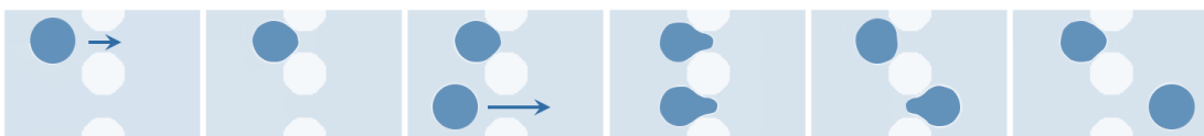
Fig. 3.11 Schematic of a numerical image series of two droplets passing through a geometry consisting of two pores. Adapted from Coelho et al. [60].
