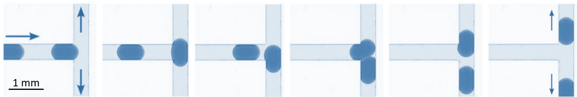
Fig. 3.6 Example of droplet collisions governing transport at a T-junction. The second droplet travels to the right as a consequence of the collision at the T-junction, regardless of the resistances of the channels downstream. Experimental images were taken with a constant time interval of 1/12 s. Adapted from Cybulski et al. [69].
