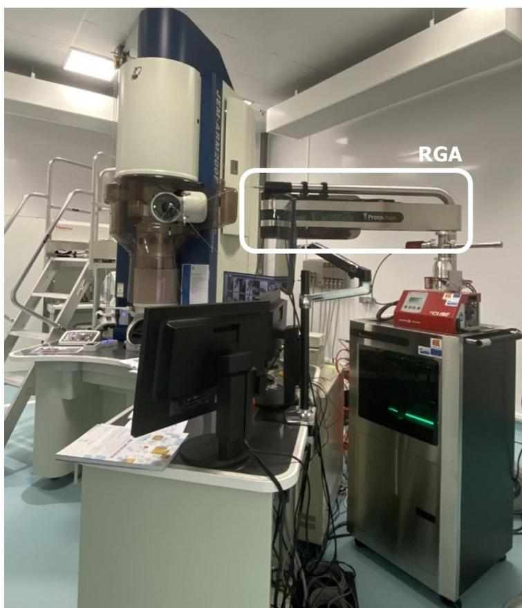
**Figure 2.13:** The Environmental Cell system coupled with the Residual Gas Analyzer from Protochips ®.
