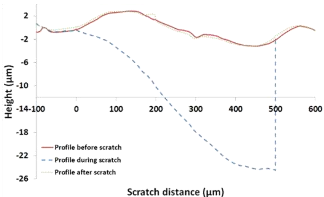
Figure 41. Height profile before, during, and after a scratch on POM-AQ based coating on a steel substrate. Complete recovery of the sample after scratch confirms the elastomeric behavior and evidences a good adherence and resistance of the coating to fracture.
