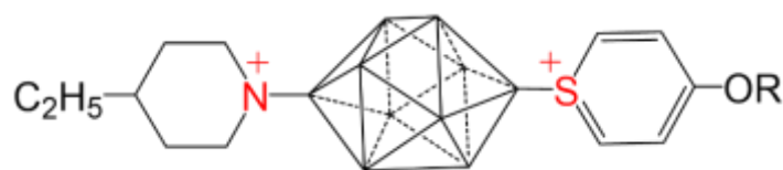
Figure 53. Hetero-(1,10)-disubstituted sulfonium and pyridinium derivative of closo -decaborate anion for liquid crystals.
