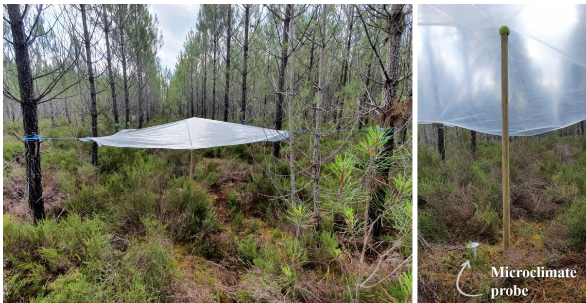
Figure 25 Precipitation exclusion system set up in a plot with understory removal in the dry moorland. This system was installed in all plots of the field experiment from mid-June to late September, 2021. Left panel and right panel are respectively pictures taken from outside and inside the area of precipitation exclusion (pictures by Lucie Bon).
