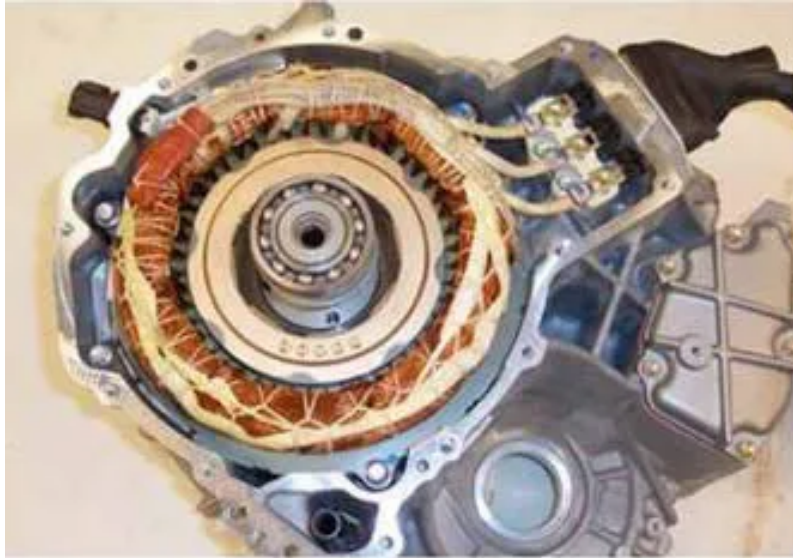
Figure 2.5: PMSM of Toyota Prius-2004 [26]
