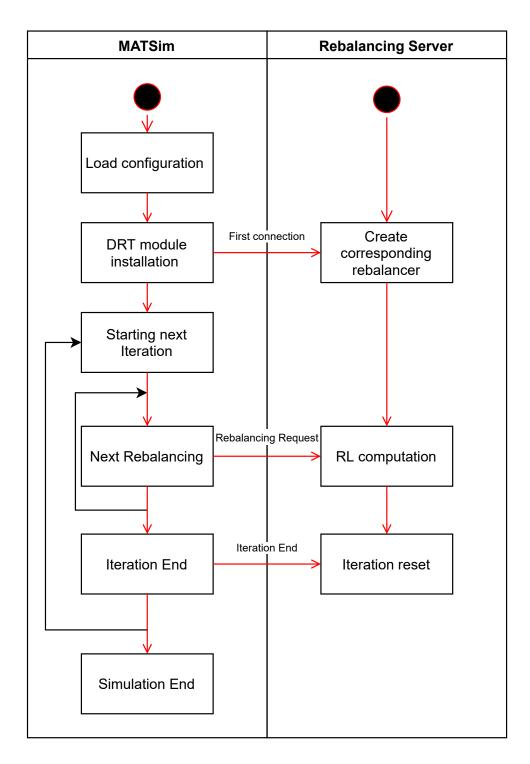
Figure 5.5: MATSim-Rebalancing server communication
