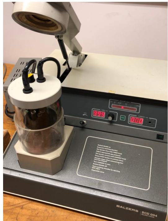
Figure 49. Preparation of hemp mortar samples (coverage with carbon)
