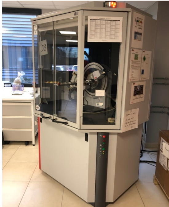
Figure 51. Bruker D8 diffractometer used for crystallography analysis
