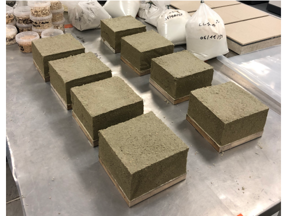
Figure 43. Hemp mortar samples laboratory drying
