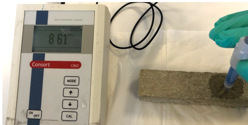
Figure 50. Measurement of the surface pH level using a WTW Sentix Sur electrode
