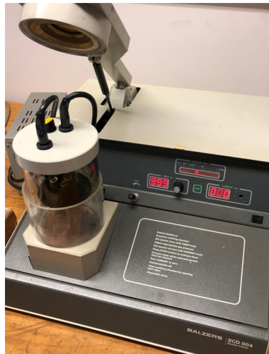
Figure 49. Preparation of hemp mortar samples (coverage with carbon)
