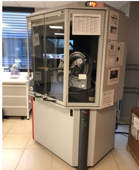
Figure 51. Bruker D8 diffractometer used for crystallography analysis
