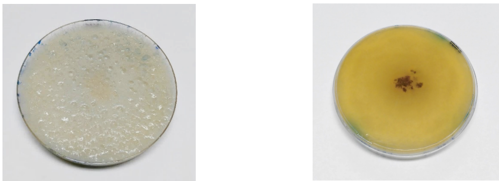
Figure 87. Image of Petri dish with isolated white fungal strain (identified as Rhizopus sp. ) after 8 days at 25 °C and 50 %RH
