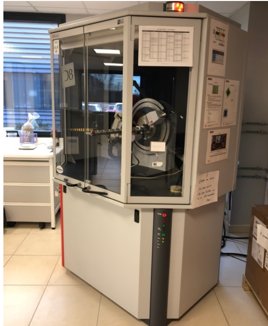
Figure 51. Bruker D8 diffractometer used for crystallography analysis
