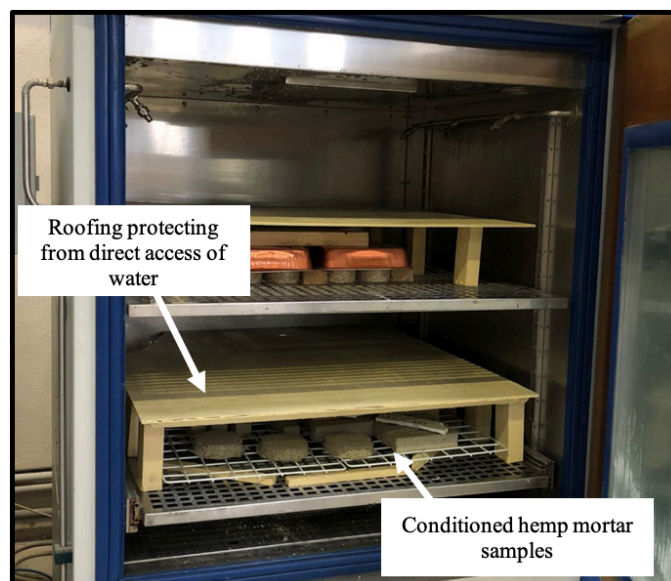
Figure 45. Disposition of the hemp mortar specimens in the climatic room before accelerated aging cycles
