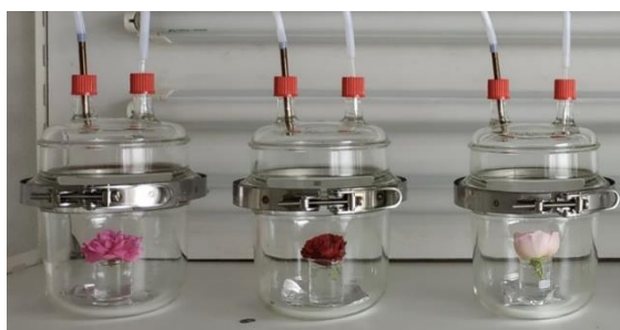
Fig. 2 – Headspace system used for the extraction of rose
