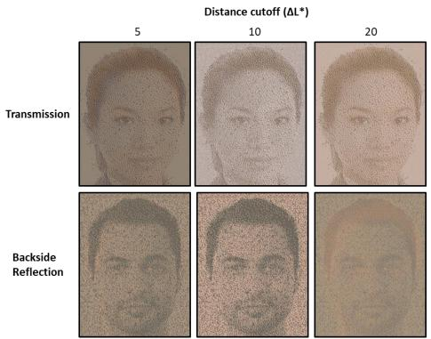
Figure 66: Comparison of two-image multiplexing solutions using two colors in transmission and backside reflection modes (four in total) using different cutoff distances of  $\Delta L^*$  (5, 10 and 20). For each cutoff distance, the simulated images in each mode of observation are displayed.
