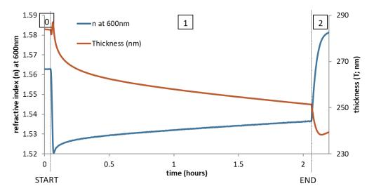
Figure 28: In-situ ellipsometric behavior of a xerogel TiO<sub>2</sub> film on Si wafer during a 2-hour thermal treatment at 130°C. The refractive index (n at 600 nm; blue curve) and the thickness (T; red curve) of the film are presented as a function of time.
