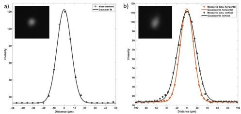
a) Spot size captured by the camera (inset) at the focal plane " $f_0$ " and the fitted gaussian profile for the vertical profile. b) Spot size captured by the camera at the plane " $f_2$ " fitted to a Gaussian profile for both vertical and horizontal profiles. Every profile was fitted with a -2r.
