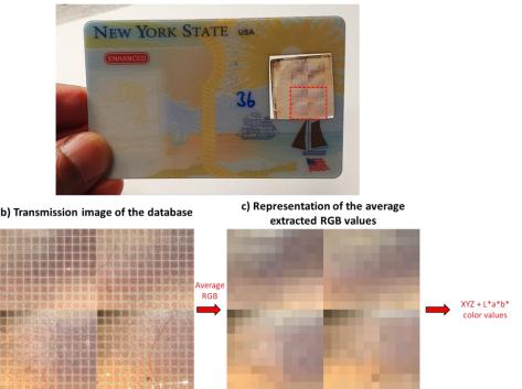
Figure 46: (a) Picture by a phone camera of the database consisting of 480 squares as highlighted in red. The image processing method for color extraction is presented. First, an image is taken of the database with the camera setup, normalized and the colors are averaged at the center of each square as delimited by the red square. The extracted sRGB values (c) are transformed to CIE XYZ values and then converted to CIE L\*a\*b\* coordinates.
