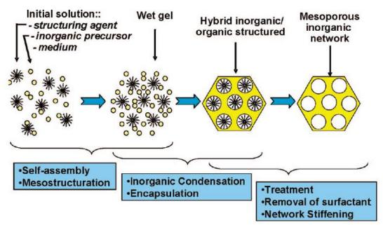
Figure 9: Schematic representation of the preparation of mesoporous materials via the EISA method adapted from Sanchez et al.<sup>40</sup>.
