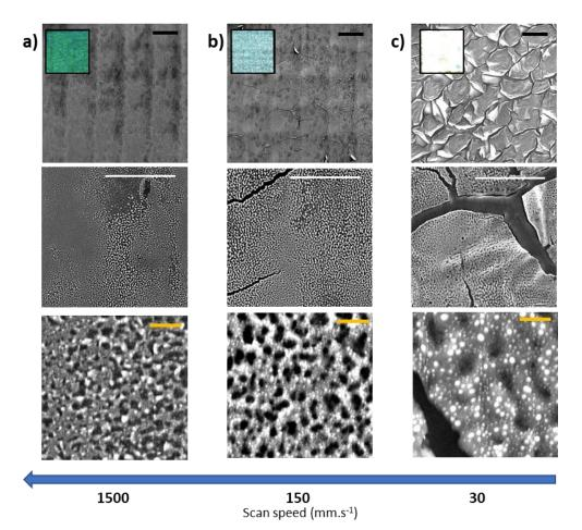
Figure 71: Investigation of surface modulations by SEM microscopy. Three nanostructures (a, b and c) were produced by using the same repetition rate and fluence (10 kHz; 68.0 mJ.cm<sup>-2</sup>) but with different scanning speeds, 1500 (a), 150 (b) and 30 (c) mm.s<sup>-1</sup>. The black scalebars of the top figures are of 50μm, the white scalebars in the middle figures are of 10 μm and the yellow scalebars of the bottom figures is of 200 nm.
