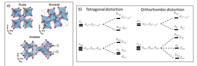
Figure 11: a) Crystal structures of TiO<sub>2</sub> rutile (tetragonal), brookite (orthorhombic) and anatase (tetragonal) polymorphs adapted from Haggerty et al.<sup>46</sup>. b) Tetragonal (anatase and rutile) and orthorhombic (brookite) distortions of TiO<sub>6</sub> result in the formation of different sub-bands in the electronic structure adapted from Tian et al.<sup>49</sup>.
