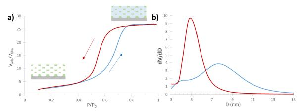
Figure 20: (a) Adsorption (blue) and desorption (red) curves a function of the relative water vapor pressure. (b) Extraction of the pore size distribution based on (a). Taken from T. Bottein thesis<sup>24</sup>.
