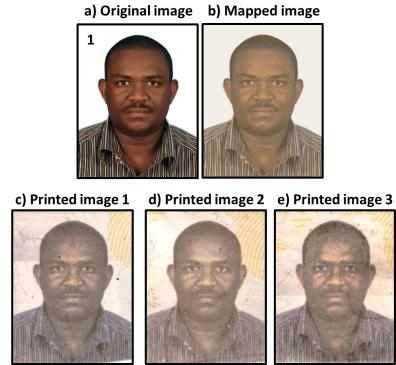
Figure 64: The original portrait (a) is gamut mapped (b) using 10 primaries in transmission mode. The resulting image is printed in three different samples (c, d and e) and detected in transmission.
