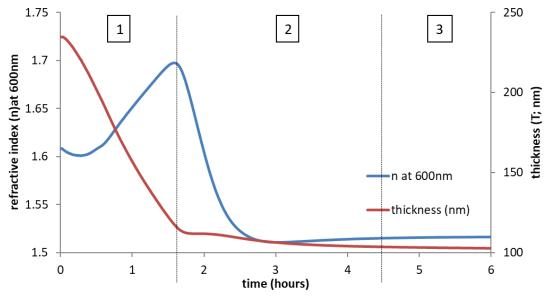
Figure 29: In-situ ellipsometric behavior of a xerogel TiO<sub>2</sub> film on Si wafer during a 6-hour 254 nm UV treatment. The refractive index (n at 600 nm; blue curve) and the thickness (T; red curve) of the film are presented as a function of time.
