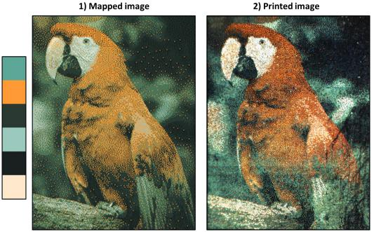
Figure 72: Full-color image printing in diffraction mode. The mapped image (1) is simulated by using 6 primaries depicted at the left of the figure. It is then vectorized and printed on a sample. The resulting image was produced by using 35x35 μm<sup>2</sup> pixels and has a real size of 10.6x13.2 mm<sup>2</sup>. The image is observed with the camera setup in diffraction mode (2).
