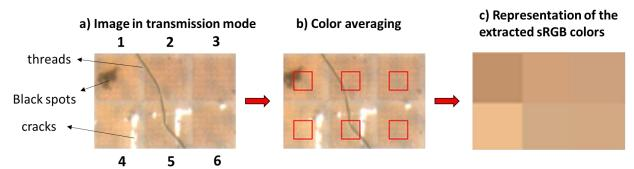
Figure 47: 6 nanostructures are printed on a PC TiO<sub>2</sub>:Ag card (a) presenting several artefacts, such as threads, black spots, holes and lamination artwork. The color averaging for each nanostructure is highlighted in a red square (b). In some cases, the presence of artefacts can hinder the color extraction, resulting in erroneous color values (c).
