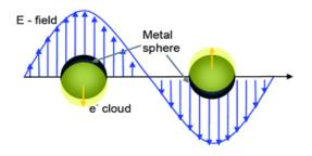
Figure 12: Schematic representation of plasmon resonance.
