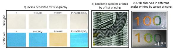
Figure 3: a) An invisible ink is deposited by flexography that reveals a fingerprint under UV light (390 nm) and is invisible under white light .<sup>4</sup> b) An example of microscale patterns printed on banknotes using offset lithography<sup>10</sup>. c) An OVD (optically variable device) is produced by screen printing magnetic crystals depicting different colors depending on the observation angle (relative angles of 5 and -15°)<sup>13</sup>.
