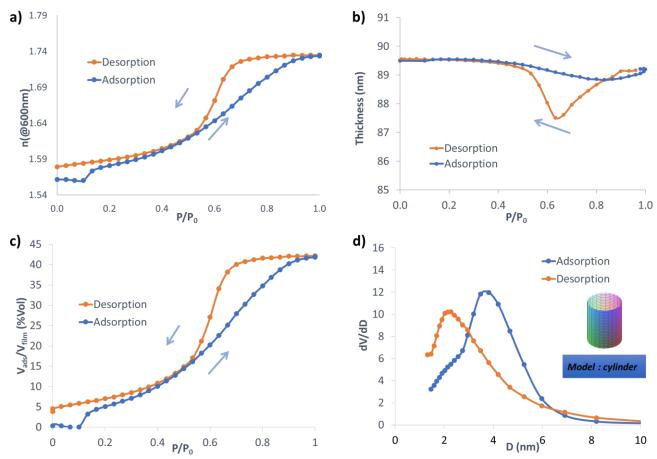
Figure 31: Adsorption-desorption isotherm of a stabilized mesoporous  $TiO_2$  film of n (a), T (b) and  $V_{ads}/V_{film}$  (c) as a function of the vapor solvent pressure (P/P<sub>0</sub>). The pore size distribution (d) is determined for a contact angle of 10° and by considering the pore shape as cylindrical as illustrated inset.
