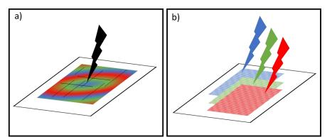
Figure 5: (a) Schematic illustration of the laser technology proposed by Lazzari et al.<sup>17</sup> where a laserable layer is carbonized to produce grey levels and mask the underlying color subpixels. (b) Schematic illustration of another laser-based technology developed by Lesur et
