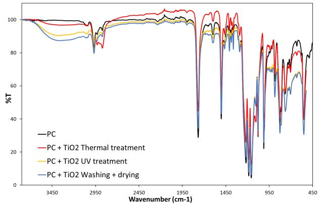
Annex 1: FTIR spectra of the evolution of a mesoporous TiO<sub>2</sub> film
