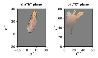
Figure 48: 2D projections of the colors of the database recorded in transmission mode. The colors are illustrated in the a\*b\* plane with the dashed black line depicting the convex hull of the points, representing the attainable colors, and in the L\*C\* plane. Each colored point represents the color of a square.
