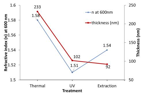
Figure 30: Summary of the ex-situ ellipsometric behavior after each stabilization step. The refractive index (n at 600 nm; blue curve) and the thickness (T; red curve) of the film are presented after each step.
