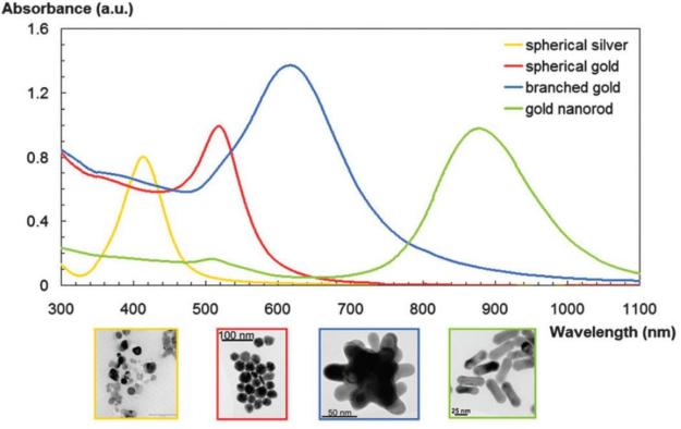
Figure 13 : Example of the plasmon resonance of metal NPs of different sizes, shapes and materials proving its dependence on all these features<sup>93</sup>.
