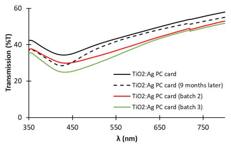
Figure 57: UV-Visible transmission spectra of TiO<sub>2</sub>:Ag PC cards. The solid black curve represents the measurements carried after laminating a TiO<sub>2</sub>:Ag PC card (batch 1) and the dotted curve represents the same sample after 9 months. Other samples prepared in the same manner are characterized and illustrated by the red and green curves, belonging to different sample batches (2 and 3).
