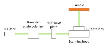
Figure 37 : Schematic representation of the nanosecond laser setup.
