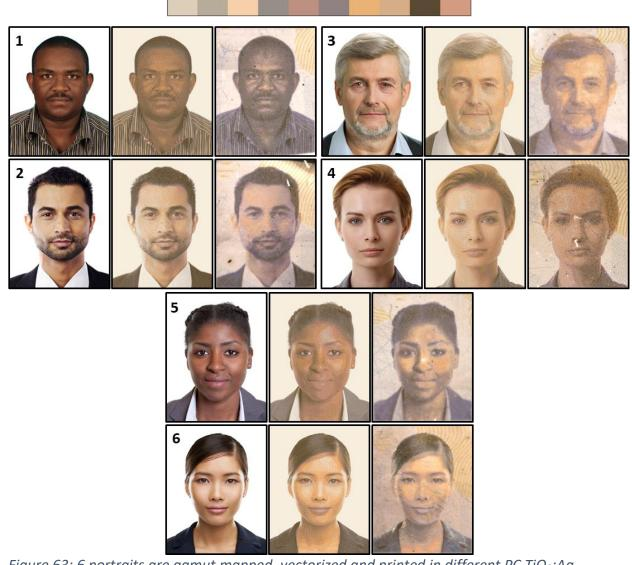
Figure 63: 6 portraits are gamut mapped, vectorized and printed in different PC TiO<sub>2</sub>:Ag cards using the 10 primaries observed in transmission mode as depicted on top of the figure. The dimensions of every printed image are 10.5x13.45 mm<sup>2</sup>.
