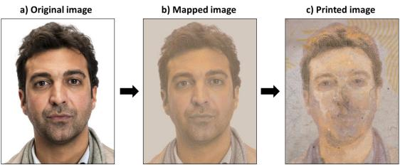
Figure 60: (a) Original image is gamut mapped in transmission mode (b), vectorized and printed on a PC TiO<sub>2</sub>:Ag card (c) depicting several printing errors.
