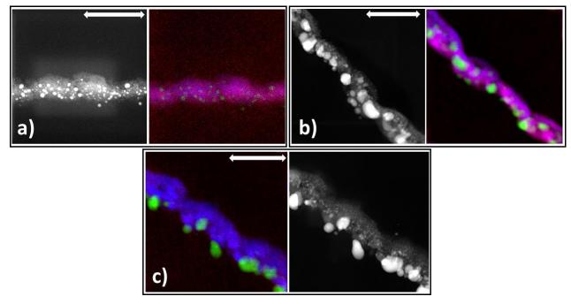
Figure 39: (a) Cross-section TEM images of the untreated TiO<sub>2</sub>:Ag film embedded in a PC card and the film laser-processed at 10 kHz (b) and at 40 kHz (3) with a laser power 28.5 mW and scanning speed of 50 mm.s<sup>-1</sup>. For each condition, the chemical mapping is illustrated on the right side where silver (green), titanium (blue) and oxygen (red) are highlighted. The scale bar represents 200 nm for every chemical mapped image.
