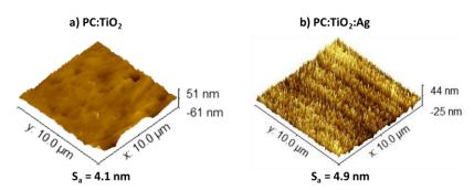
Figure 33: 3D AFM 10μmx10μm micrographs of the surface of (a) a stabilized TiO<sub>2</sub> film deposited on polycarbonate and (b) after silver impregnation and reduction.
