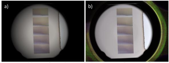
Figure 41: (a) Image of a sample taken with the same setup in "transmission" mode depicting lightness decay from the center to the borders. (4) Normalized image of the sample, correcting the lightness decay of the lens.
