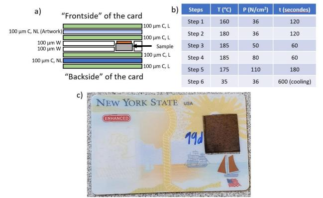
Figure 34: (a) Sketch of the card configuration with a stack of 8 PC sheets for sample lamination, (b) lamination program with 6 steps with varied temperatures, pressures and times. (c) Image taken with a camera phone of the "frontside" of a laminated card containing a 2x2cm sample.
