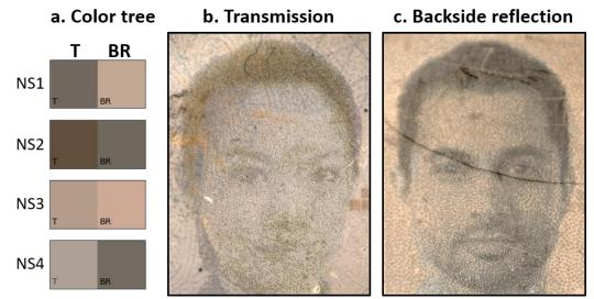
Figure 67: Experimental result of two-color image mutiplexing. The color tree (a) consists of 4 nanostructures (NS1 to NS4) depicting different colors in transmission (T) and backside reflection (BR). The multiplexed image is printed and characterized with the camera setup in transmission (b) depicting a woman and in backside reflection (c) depicting a man.
