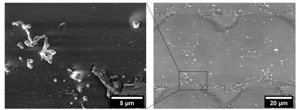
Figure 68: SEM images of a laser-processed PC:TiO<sub>2</sub>:Ag film depicting severe delamination of the material.
