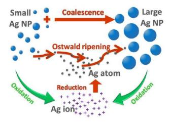
Figure 15: Illustration of the main mechanisms that control the size distribution of AgNPs embedded in a TiO<sub>2</sub> host matrix when irradiated by laser<sup>94</sup>.
