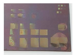
Figure 38: Image taken by a phone camera of laser inscriptions made at the focal plane  $f_0$  on a TiO<sub>2</sub>:Ag PC card presenting bubbles due to intense irradiation.
