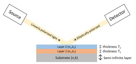
Figure 19: Schematic representation of an ellipsometer.
