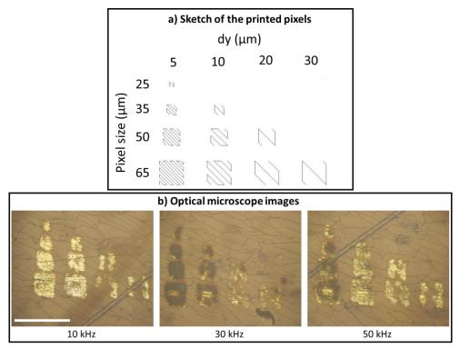
Figure 44: (a) Design of pixels with different sizes (25-65  $\mu$ m) and different dy values (5-30 $\mu$ m). These pixels were printed in a PC:TiO<sub>2</sub>:Ag card at three different repetition rates (10,
