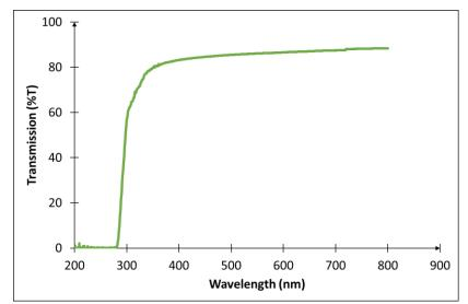
Figure 22: UV-Vis transmission (%T) spectra of a PC substrate between 200 and 800 nm wavelength.
