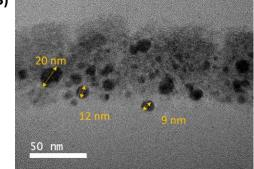
Figure 35: (a) Optical microscope image of a PC TiO<sub>2</sub>:Ag card after lamination presenting slight cracking. (b) UV-Vis spectral curves of the sample before (in blue) and after lamination (in orange). (c) STEM image of the cross section of PC TiO<sub>2</sub>:Ag card depicting small AgNPs with diameter ranging from 5 to 20 nm in the titania matrix.
