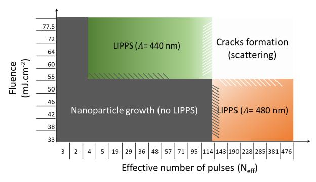
Figure 73: Parameters regime of laser-induced surface modifications of a database of 480 unique sets of parameters with varied fluences (20-74 mJ.cm<sup>-2</sup>) and effective number of pulses (2-476).
