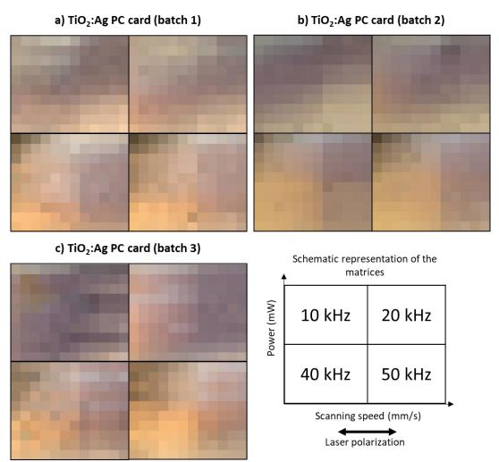
Figure 58: The database was printed in three different samples belonging to three different sample batches (a, b and c). The colors were characterized in transmission and represented in a 2D projection following the scheme.
