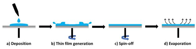
Figure 8: Schematic representation of the four main steps of spin-coating. (a) The sol is deposited on top of the substrate correctly placed on the spinner. (b) Then the film is rotated at constant speed spreading the sol on the surface by centrifugal force (spin-up). (c) Governed by the viscosity of the solution, the thickness of the formed film gradually decreases (spin-off). (d) In the final part of the spin-coating, the solvent is evaporated, reducing even more the thickness of the film.
