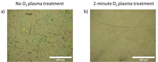
Figure 26: Optical microscope images of the surface of a PC:TiO<sub>2</sub> substrate untreated (a) and treated with an oxygen-plasma treatment for 2 minutes (b).
