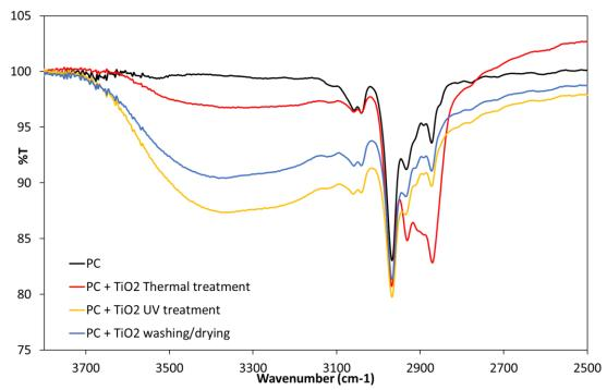
Figure 27: FTIR-ATR spectra measurements of the evolution of a TiO<sub>2</sub> film over the course of the stabilization process. The thermal, UV and washing steps are illustrated by the red, blue and yellow curves respectively. The black curve is related to a virgin PC substrate.
