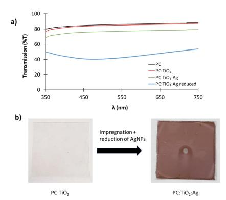
Figure 32: UV-Visible transmission spectrum (a) of a virgin PC substrate (black), a mesoporous TiO<sub>2</sub> film on PC (red) which was then impregnated with silver ions (green) and reduced by UV exposure (blue). The PC:TiO<sub>2</sub> sample is initially transparent (b) and gains a brownish color after the impregnation of silver salts and their reduction to silver nanoparticles.
