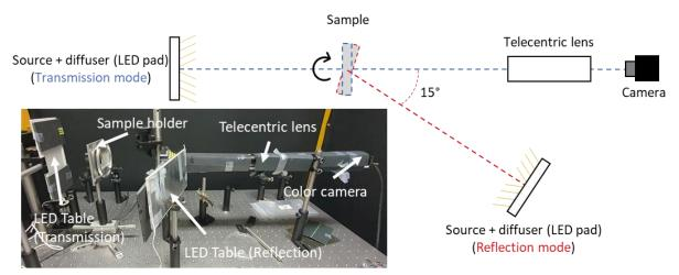
Figure 40: Sketch and picture of the image acquisition setup.
