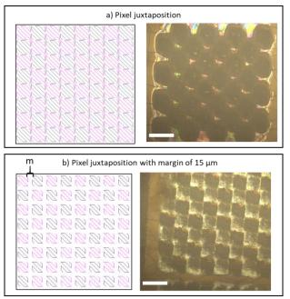
Figure 45: (a) A 400x400  $\mu$ m<sup>2</sup> square containing 8x8 50 $\mu$ m<sup>2</sup> binary pixels is inscribed in a TiO<sub>2</sub>:Ag PC card and observed under the microscope depicting severe pixel overlapping. (b) Introducing a margin of 15  $\mu$ m between the pixels and reducing their size to 35  $\mu$ m results in a homogenous inscription as no overlapping was observed. The scale bar of the images is 100  $\mu$ m.
