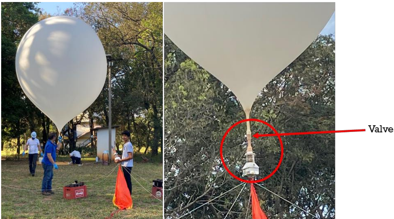
Figure 4.5: Preparation of the aerosol sampler flight (left). Zoom on the radio-controlled valve used to reduce the ascent inside the HTHH plume on 08/12.
