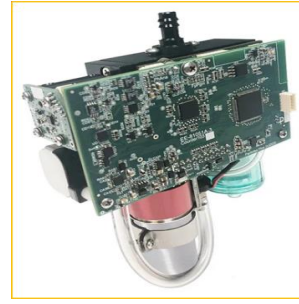
(c) A small balloon-borne OPC payload was deployed based upon the adaptation of the Particle Plus 8306 OPC profiler to make aerosol concentration measurement at eight radii between 0.15 to 5\text{ }\mu\text{m} up to the middle stratosphere (POPC). The New POPC is a similar instrument (9301 series) with 30 channels between 0.15 to 5\text{ }\mu\text{m} .
