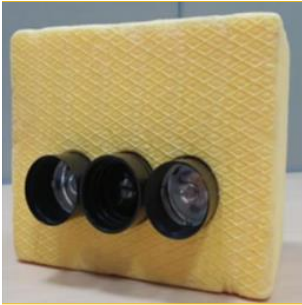
(d) Compact Optical Backscatter Aerosol Detector (COBALD). COBALD is a lightweight ( 540\text{ g} ) instrument that consists of two high-power light-emitting diodes (LEDs) that emit about 500\text{ mW} of optical power, at wavelengths of 470 and 940\text{ nm} , respectively. The backscattered light from the molecules, aerosols, or ice particles is recorded by a silicon photodiode using phase-sensitive detection. Absolute error interval of 5\% , while precision along the profile is better than 1\% in the UTLS region (Vernier et al. 2015).
