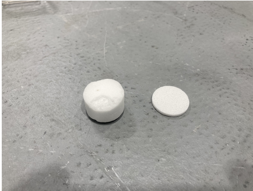
Figure 5.16 – Salt pellets before (on the left) and after grinding (on the right) to fit in the pellet holder.
