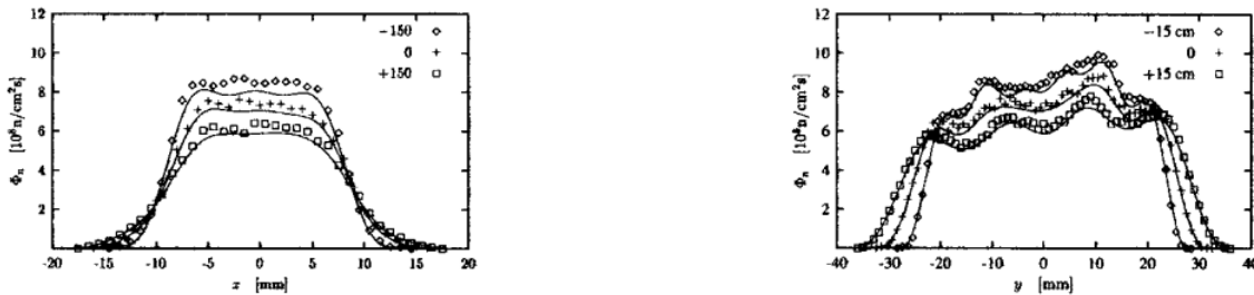
Figure 3.3 – This figure, coming from the original paper, shows the beam shape along either the x or y -axis.
