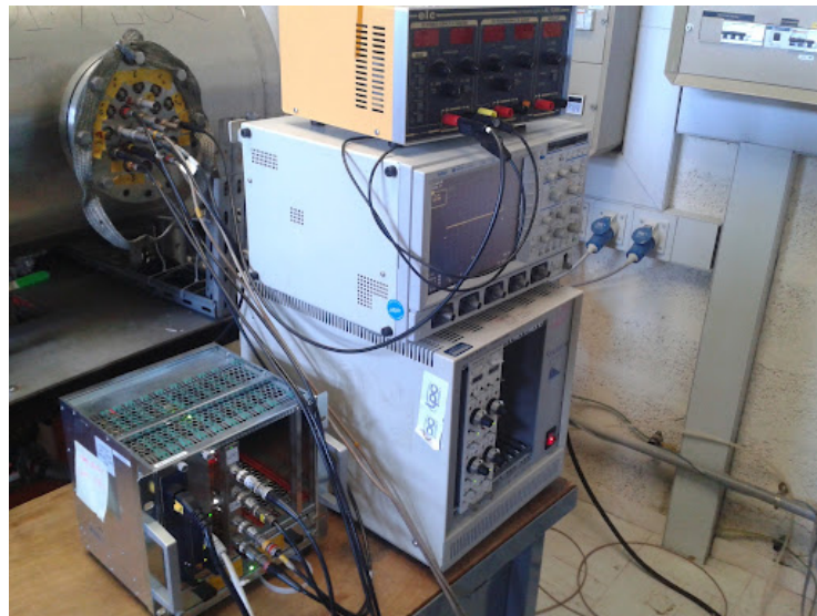
Figure 7.5 – Picture of the experimental setup used for the data acquisition of the phoswich at LPC Caen. The detector's voltages are set at 830 V by the ISEG power supply shown in the picture. The detector signals are brought to the outside with the help of the pins connector on the left of the chamber.
