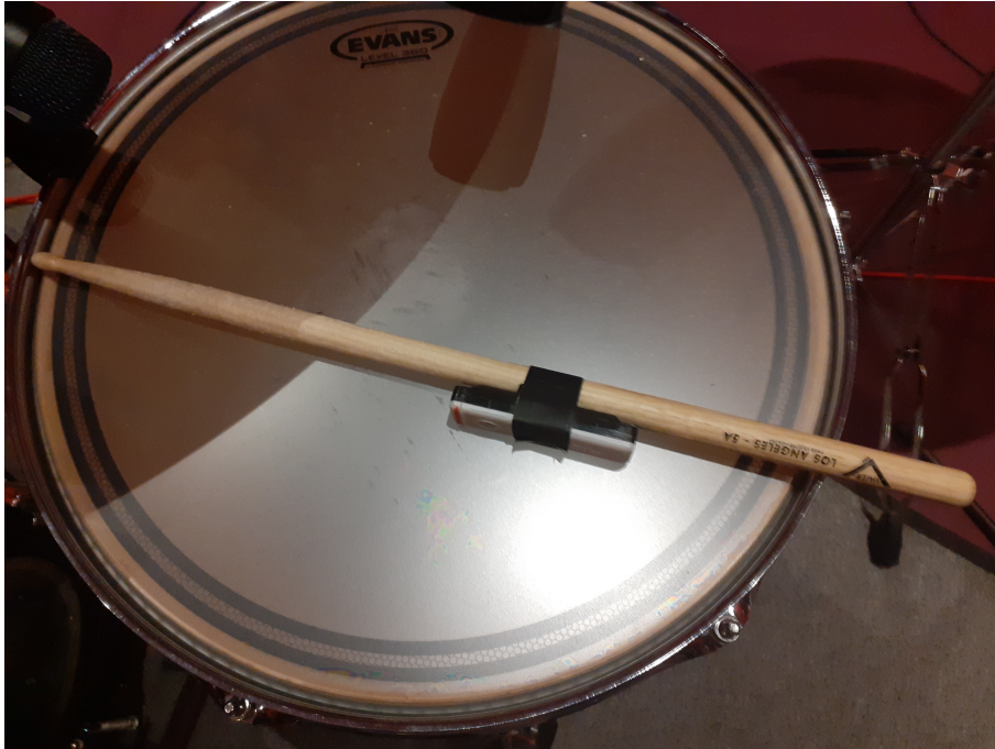
Figure 3.1: Redison Senstroke sensor mounted on a Vater 5A drumstick.
