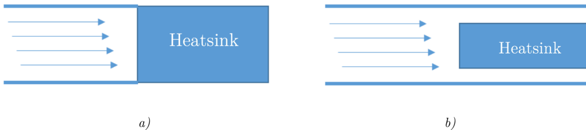
Figure 149: a) The chosen heatsink geometry and air-flow configuration - b) another common example of configuration which is not used in our study
