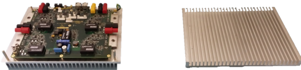
Figure 77: Natural Convection device for the Cooling Evaluation
