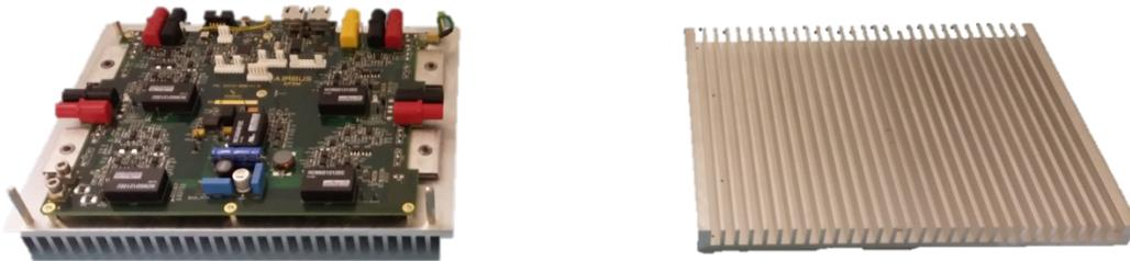
Figure 77: Natural Convection device for the Cooling Evaluation
