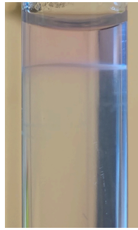
Figure 2.8: MTB culture medium showing a band of MTB growing at the oxic-anoxic interface (pink-transparent transition).
