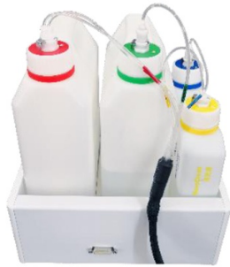
Figure 3: Reagent containers & Tubing Connections
