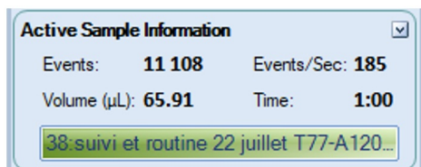
Figure 11: Active Sample Information: running information are visible during acquisition.
