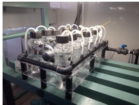
Figure 3: Low Intervention Culture System (LICSy) developed for the conservation of P. palmata strains (left). A) Schematic drawing of the LICSy. B) Picture of the collection of 120 strains of P. palmata in culture in the LICSy (right). C) Detailed picture on two rack systems fitting 12 bottles containing strains from a given population.
