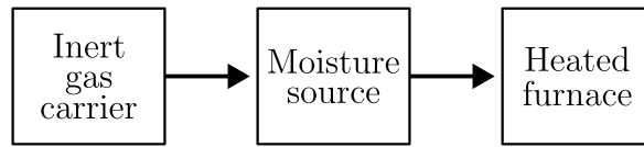
Figure 3.7: Schematic of basic wet thermal oxidation system.
