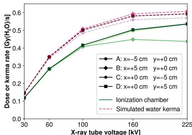
**Figure 9.** Dose rate measured by the ionization chamber (solid line) and simulated water kerma rate (dashed line) at five tube voltages and four points in a radius of 5 cm around locations corresponding to the center of the irradiated OFs.
