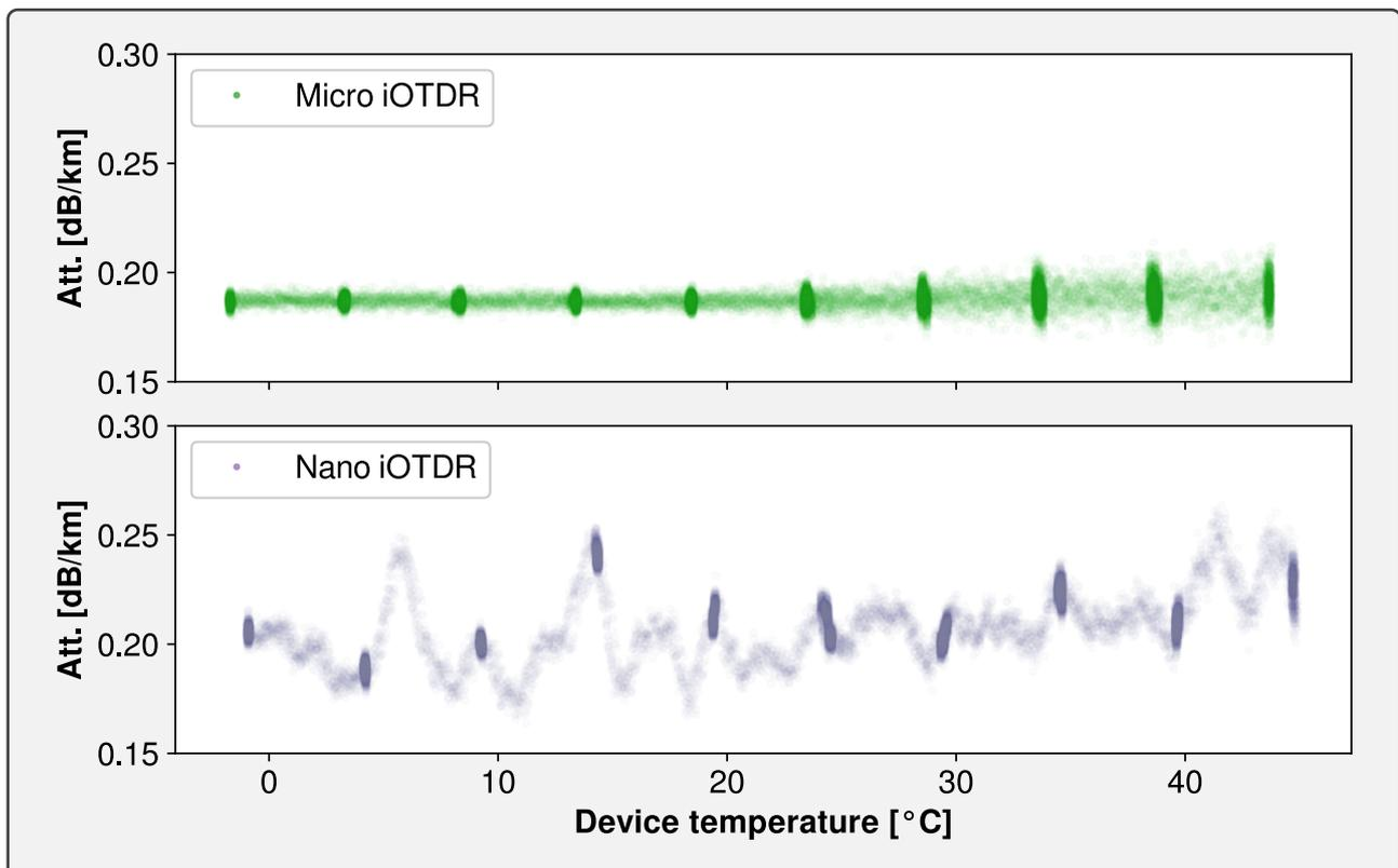
**Figure 3.14.** – Measured attenuation as a function of device temperature, for all acquired data on Micro and Nano iOTDR devices.
