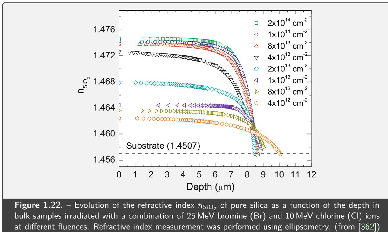
is linked to a change of the material refractive index, which has been evidenced under irradiation with particles of many different natures, such as X-rays [357],  $\gamma$  rays [358], protons [359], neutrons [360] and ions [361, 362]. An example is shown in **Figure 1.22** with measurements of the refractive index of pure silica irradiated at different heavy ion fluences.
