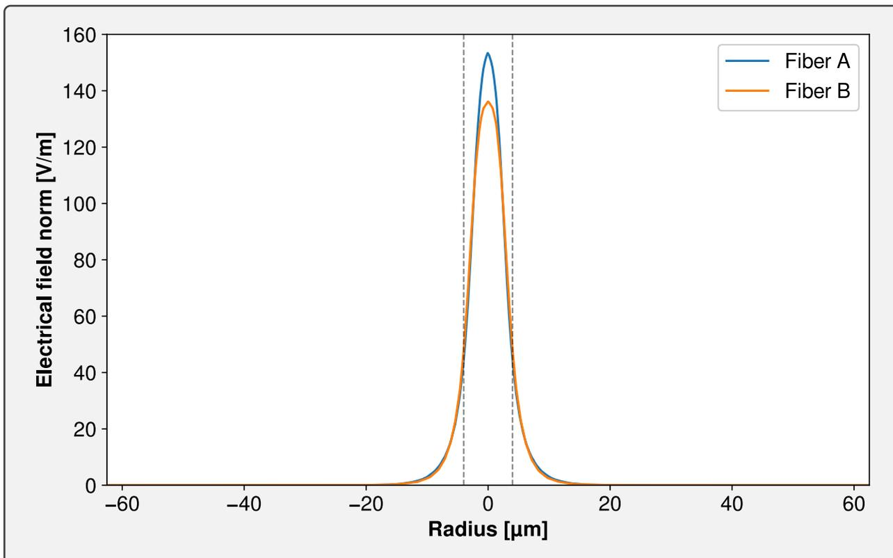
Figure 2.2. – 1D mode profile at  $\lambda = 1610$  nm of both A- and B-type fibers, simulated by COMSOL. The dashed lines delimit the core area.
