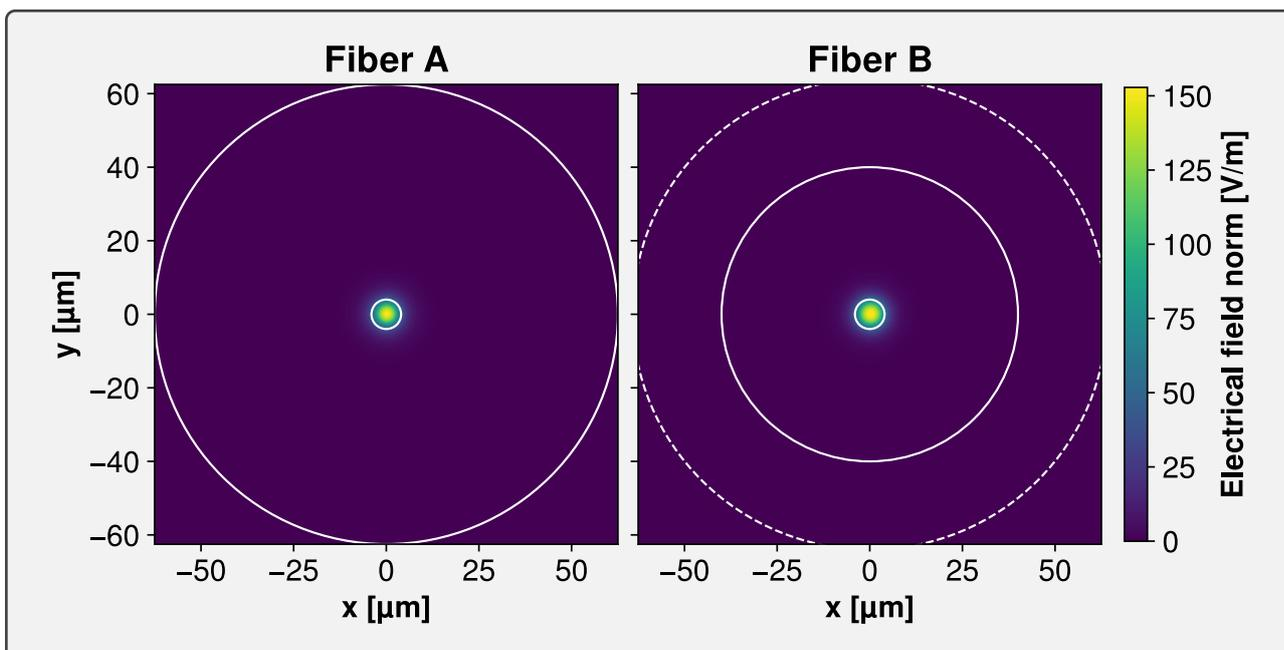
Figure 2.3. – 2D mode profile at  $\lambda = 1610$  nm of both A- and B-type fibers, simulated by COMSOL. Inner and outer white solid circles delimit core and cladding areas, dashed circle the coating area.
