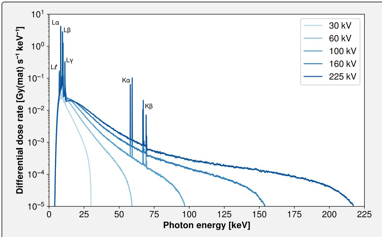
**Figure 4.14.** – Simulated differential dose response spectrum in the core of fiber **A** irradiated under X-ray with different tube voltages. The main tungsten characteristic X-ray lines are also annotated.
