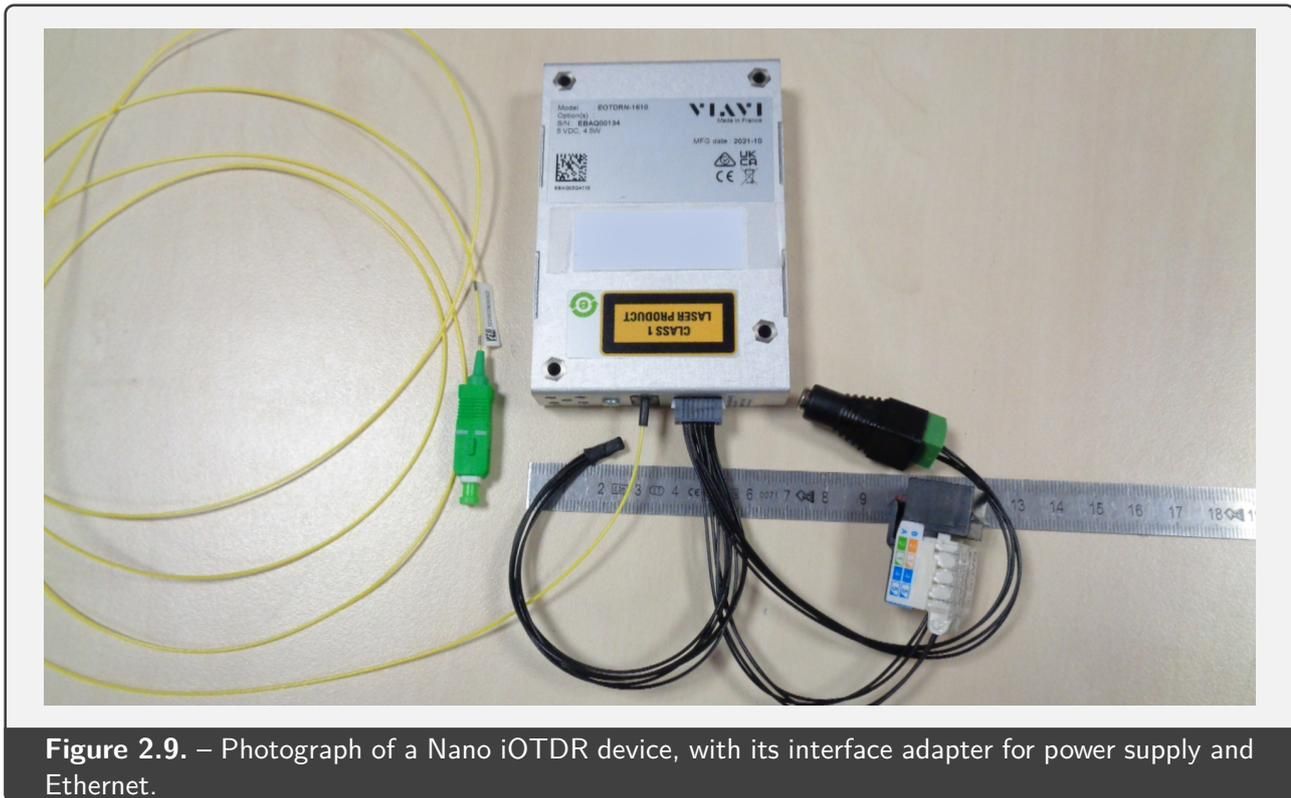
**Figure 2.9.** – Photograph of a Nano iOTDR device, with its interface adapter for power supply and Ethernet.
