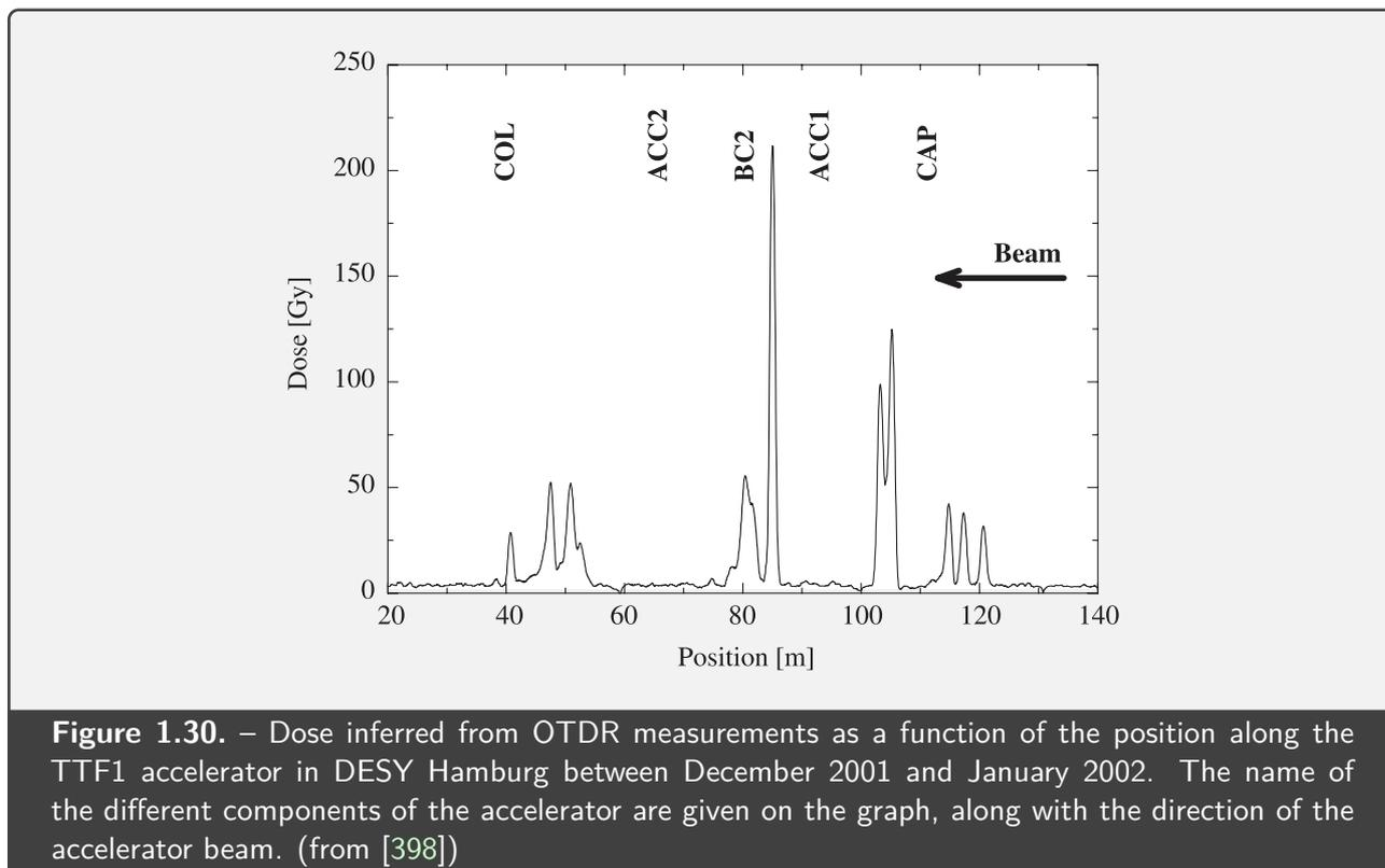
The distributed dosimetry setup involved an a high-accuracy, table-top OTDR device (Tektronix FiberMaster TFP2A), able to reach pulse widths down to 1 ns. The instrument was operated at a wavelength of 850 nm, selected because of its higher radiation sensitivity than infrared wavelengths (cf. [Section 1.2.4](#)), and a pulse width of 3 ns, to reach a good compromise between spatial resolution and measurement dynamics (cf. [Section 1.3.2](#)) [398].
