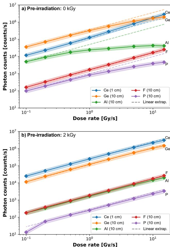
Fig. 10. Comparison of the mean value of RL signal of all tested fiber samples at different dose rates. Dashed lines show linear extrapolations from the first measurement points, in order to evaluate visually the linearity of each curve. (a) Results of the first run without preirradiation. (b) Results of the third run, totaling a preirradiation dose of  $\sim 2$  kGy. Filled areas show the uncertainty range of  $\pm 25\%$ .
