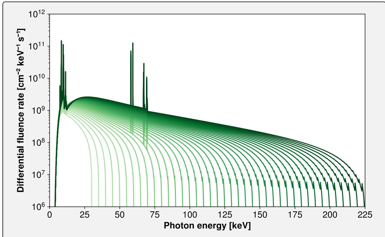
**Figure 4.10.** – SpekPy simulated spectra of X-rays irradiating an optical fiber coil placed around the beam maximum at a position  $y = 0$  and  $z = 42.5$  cm. The 40 investigated voltages between 30 kV and 225 kV are illustrated here.
