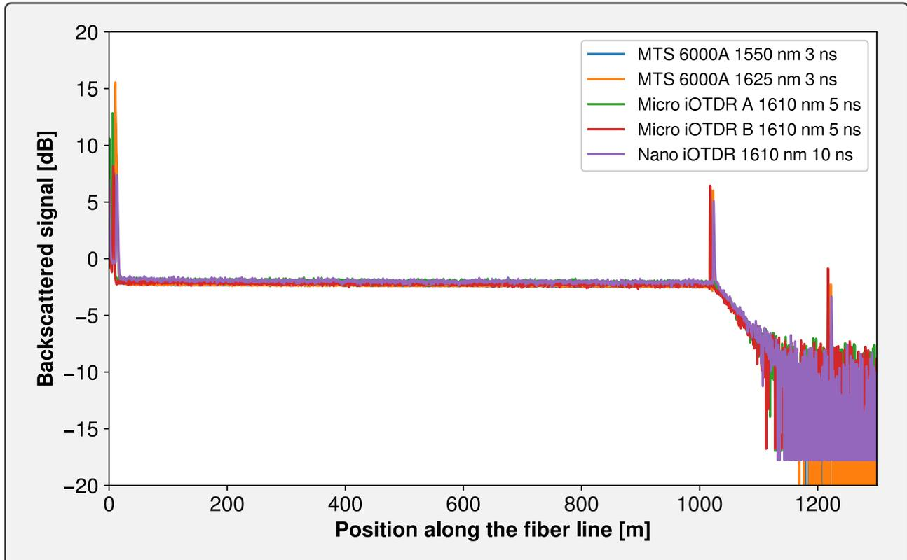
Figure 3.2. – Sample data for the metrological characterization of investigated OTDR devices. Device name, wavelength and pulse width are shown in the legend, and the common scan time was 10 s.
