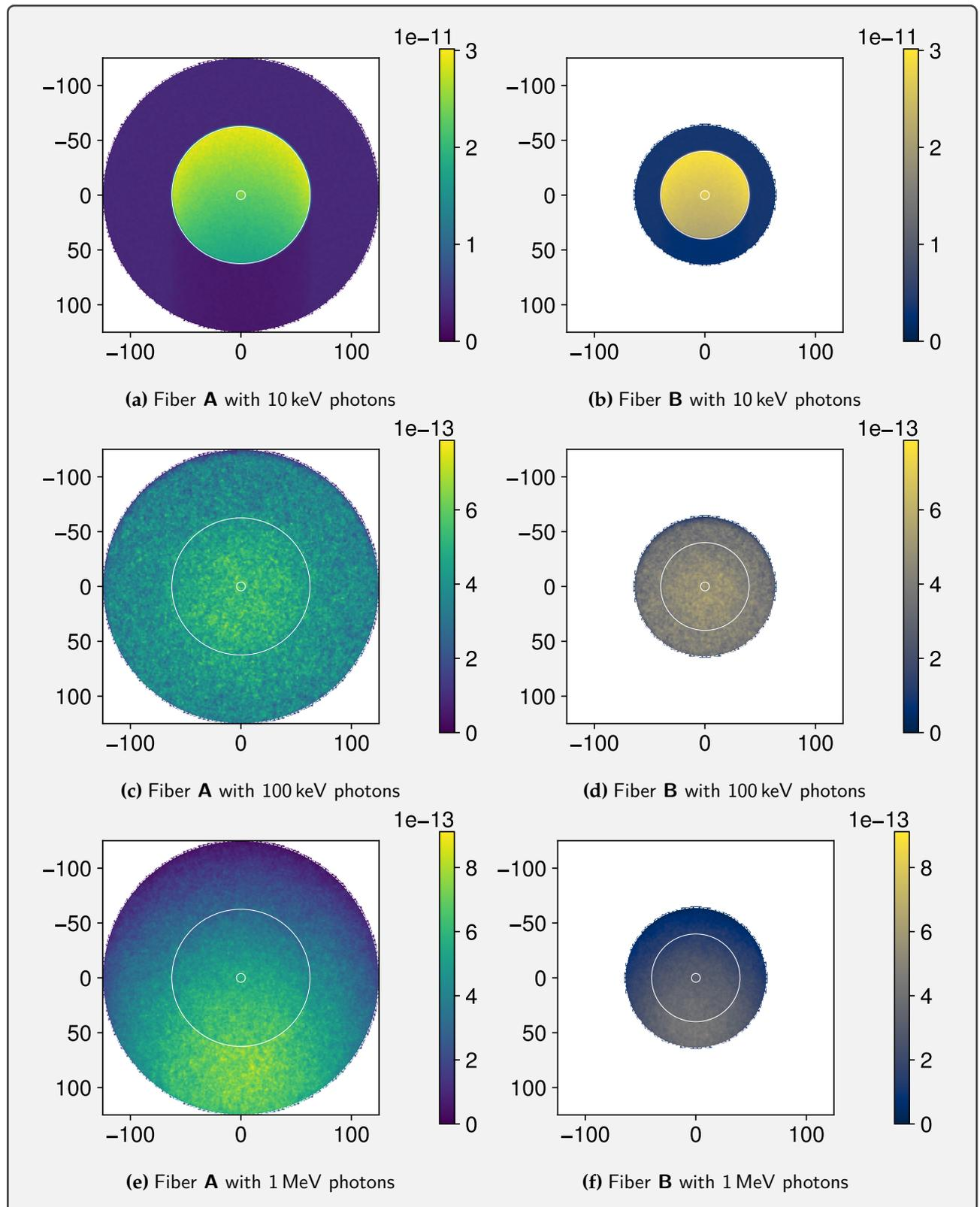
**Figure 4.5.** – Two-dimensional dose/fluence maps (in  $\text{Gy}(\text{mat})\text{cm}^2$ ) for fibers **A** and **B** irradiated with monoenergetic photons of different energies. Dimensions ( $x$  horizontally and  $z$  vertically) are in  $\mu\text{m}$ , and photons are incoming from above, i.e. toward positive  $z$  values. White circles delimit the coating (dashed lines), cladding and core areas.
