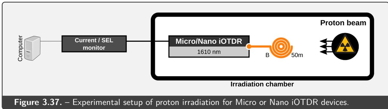
Figure 3.37. – Experimental setup of proton irradiation for Micro or Nano iOTDR devices.
