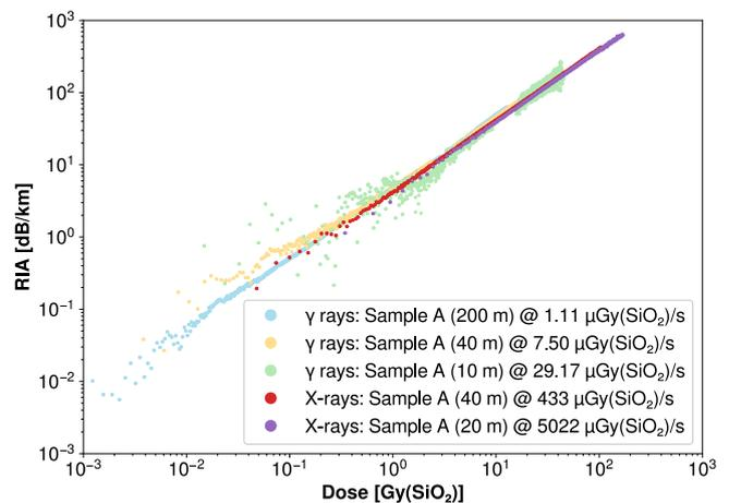
Fig. 5. Log-log plot of the compared evolution of RIA (at 1610 nm) of sample A according to dose, at different dose rates under  $\gamma$ - and X-rays.  $\gamma$  rays data are displayed in a lighter color in order to emphasize X-ray data.
