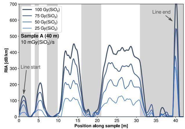
Fig. 6. Evolution of RIA measurement under X-rays (10 mGy(SiO<sub>2</sub>)/s) over the length of a 40-m sample of OF A, with portions successively shielded and unshielded to show the spatially-resolved character of the measurement. Grayed areas show the approximate locations of shielded segments.
