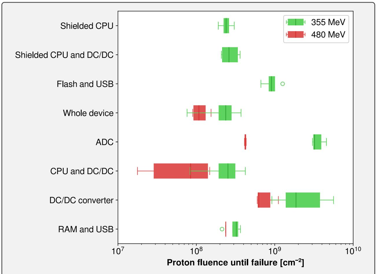
**Figure 3.39.** – Box plot of proton fluences until failure of the Micro iOTDR, according to the targeted components. Results obtained at different proton energies are shown with different colors. Circles indicate outlier data.
