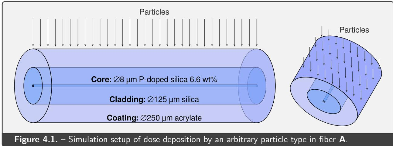
Figure 4.1. – Simulation setup of dose deposition by an arbitrary particle type in fiber A.
