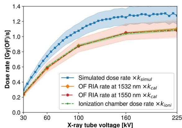
**Figure 10.** Comparison between dose rate determined by three different means: simulation, scaling of RIA rate and scaling of ionization chamber measurements; for X-ray tube voltages between 30 kV and 225 kV. Filled areas show uncertainties at  $\pm 2\sigma$ .
