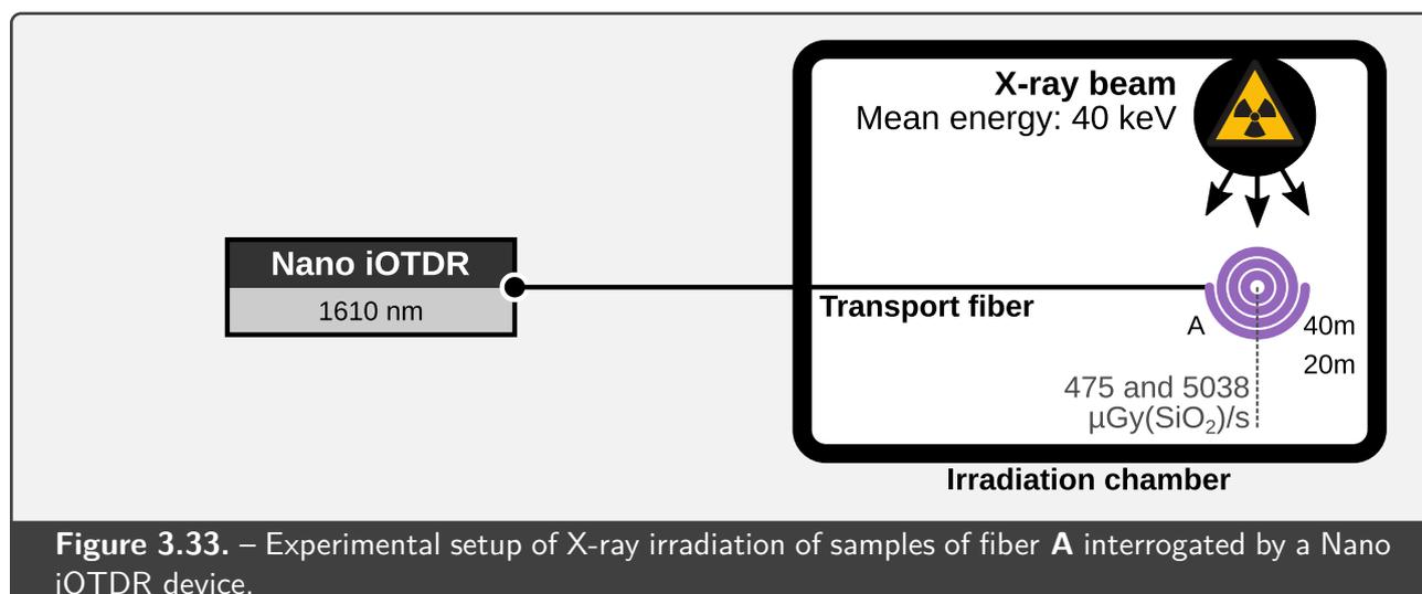
**Figure 3.33.** – Experimental setup of X-ray irradiation of samples of fiber A interrogated by a Nano iOTDR device.
