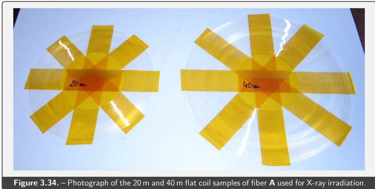
**Figure 3.34.** – Photograph of the 20 m and 40 m flat coil samples of fiber **A** used for X-ray irradiation.
