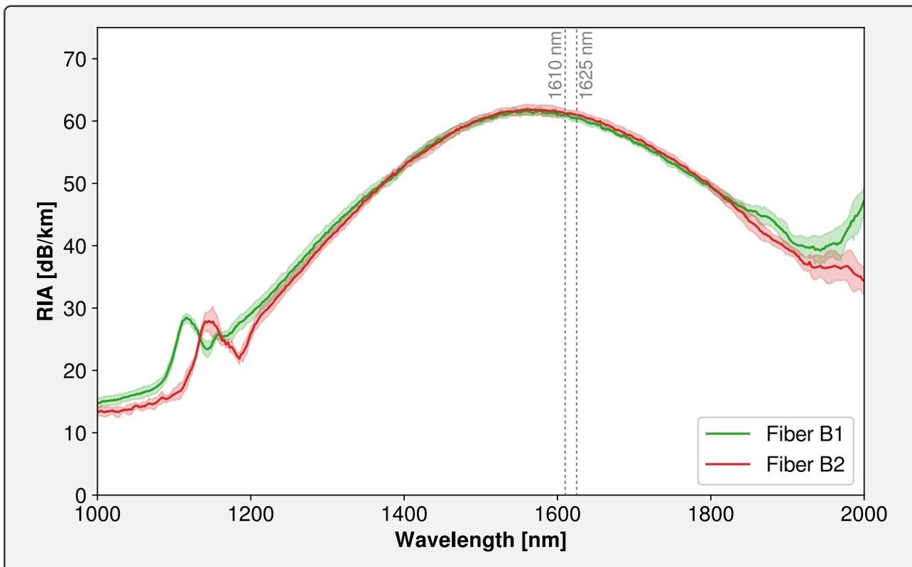
**Figure 3.27.** – Spectral RIA, in the near-infrared domain, of the **B1** and **B2** samples irradiated under  $\gamma$  rays at a dose of 12.9 Gy(SiO<sub>2</sub>). Filled areas in lighter color show uncertainties at  $\pm 2\sigma$ . Position of wavelengths 1610 nm and 1625 nm are indicated in dashed lines for further reference.
