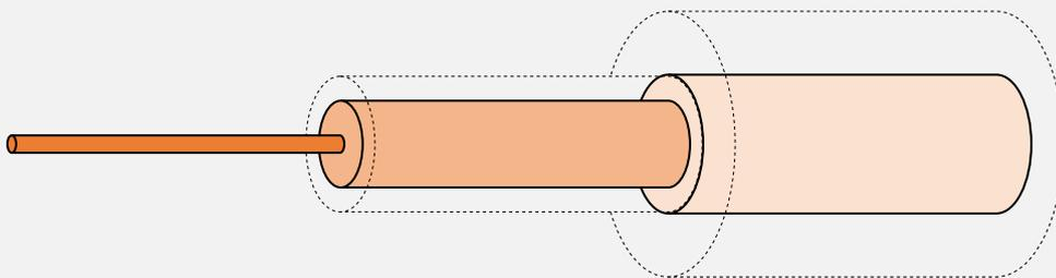
**Figure 2.1.** – Section view of the **B** fiber (in solid lines), compared to the same scale with fiber **A** (represented in dashed lines).
