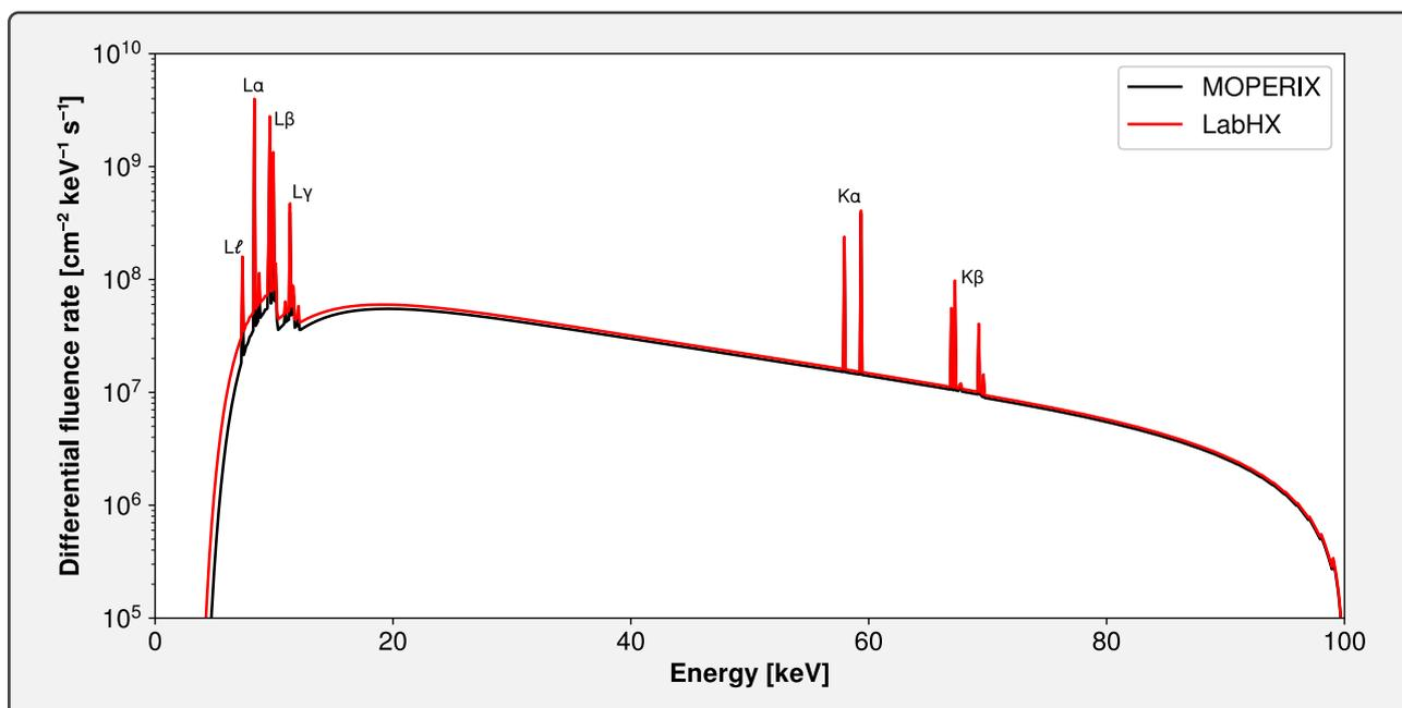
**Figure 2.12.** – SpekPy simulated fluence rate spectra of MOPERIX and LabHX X-ray tubes operated at a voltage of 100 kV and a current of 1 mA, from a location at a distance of 50 cm vertically from the anode center. Filtering from the beryllium window (different for each irradiator) and from the air layer are taken into account. The main tungsten characteristic X-ray lines [511] are also annotated.
