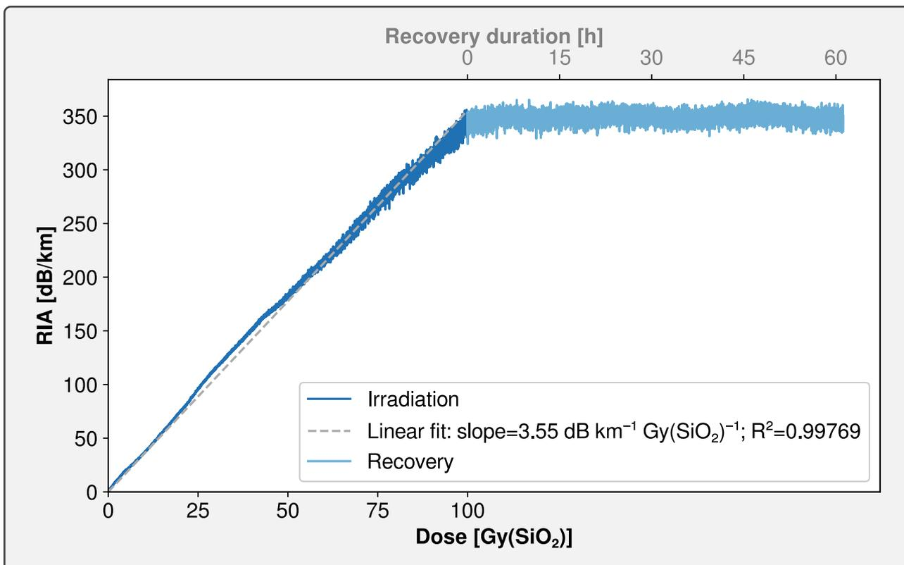
**Figure 3.35.** – Evolution of 1610 nm RIA of fiber **A** irradiated under X-rays at 475  $\mu\text{Gy}(\text{SiO}_2)/\text{s}$ . Recovery data are indicated in a lighter color. Dashed line indicates the linear fit applied to RIA data during irradiation.
