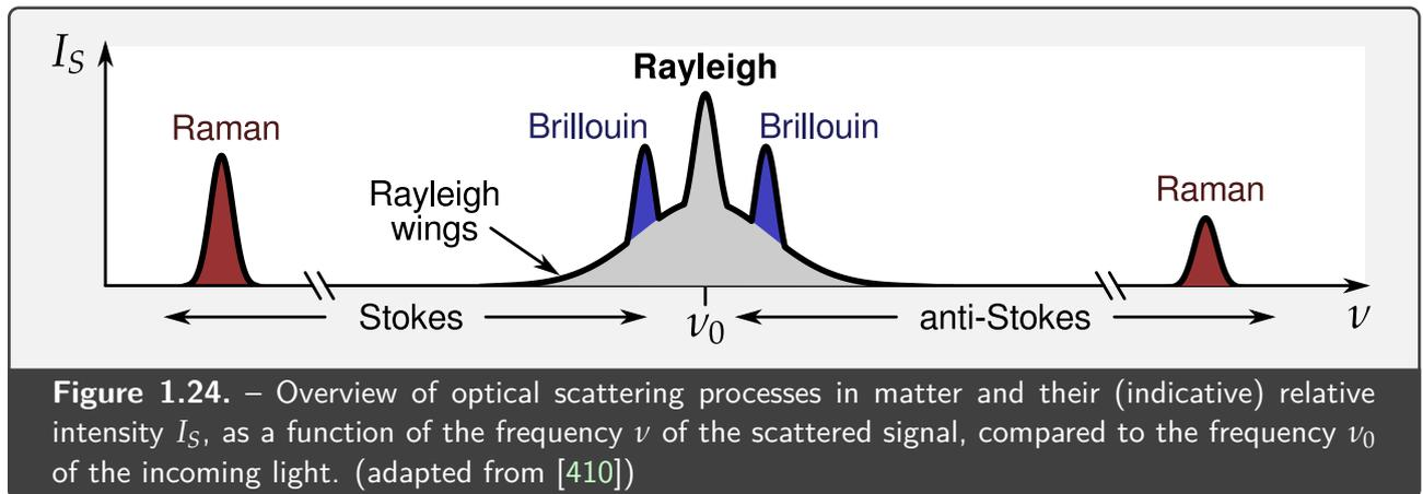
These local perturbations come from various origins, that each produce a distinguishable scattering process, as illustrated in **Figure 1.24**.
