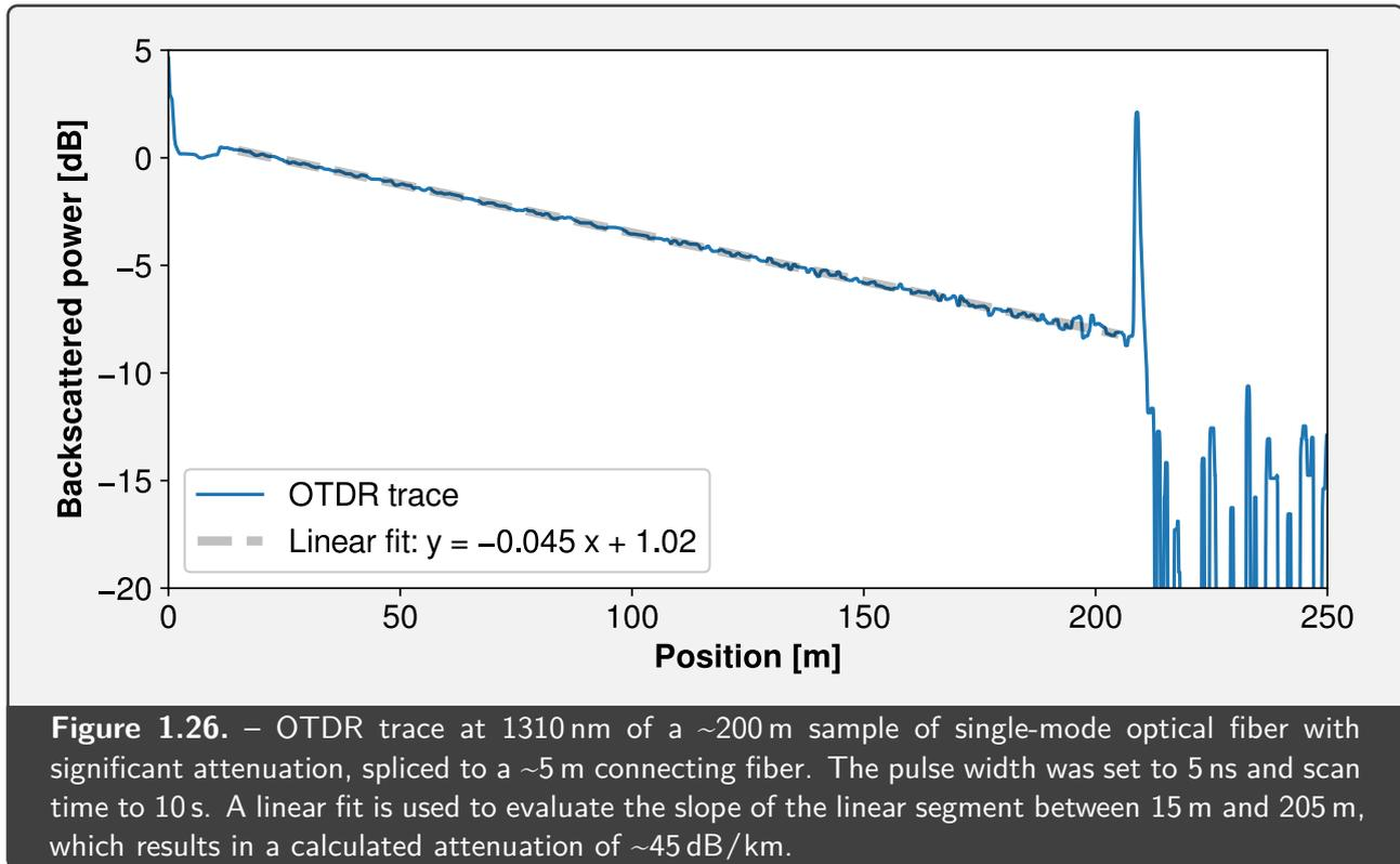
**Figure 1.26.** – OTDR trace at 1310 nm of a ~200 m sample of single-mode optical fiber with significant attenuation, spliced to a ~5 m connecting fiber. The pulse width was set to 5 ns and scan time to 10 s. A linear fit is used to evaluate the slope of the linear segment between 15 m and 205 m, which results in a calculated attenuation of ~45 dB/km.
