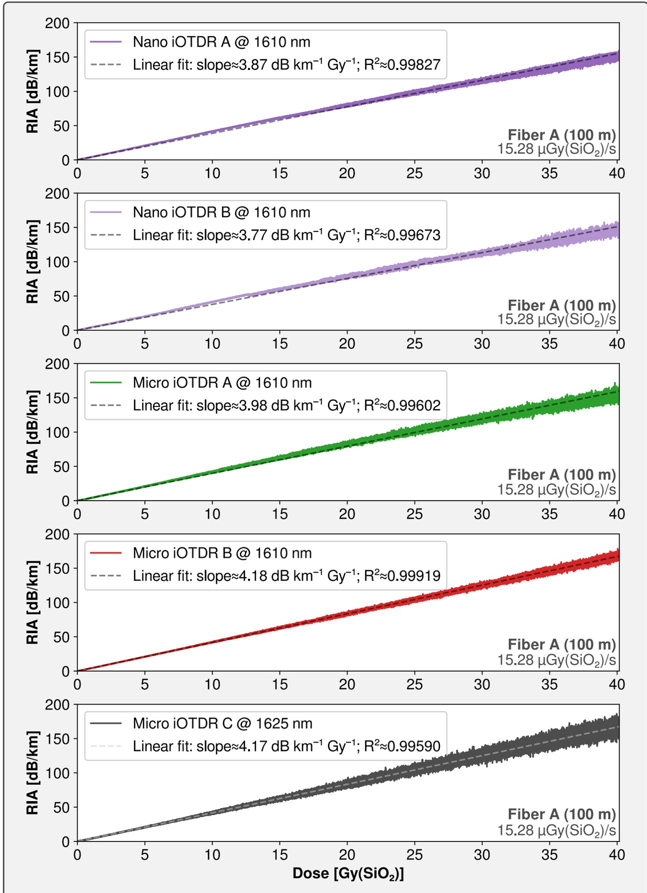
Figure 3.32. – RIA as a function of dose, measured on 100 m samples of fiber A with five different interrogating devices. Each data set includes a linear fit shown in dashed line.
