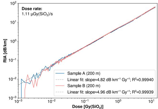
Fig. 4. Log-log plot of the compared evolution of RIA (at 1610 nm) of samples A and B according to dose at a  $\gamma$  ray dose rate of 1.11  $\mu$ Gy(SiO<sub>2</sub>)/s. A linear fit is applied on each set of results to retrieve the sensitivity of each fiber.
