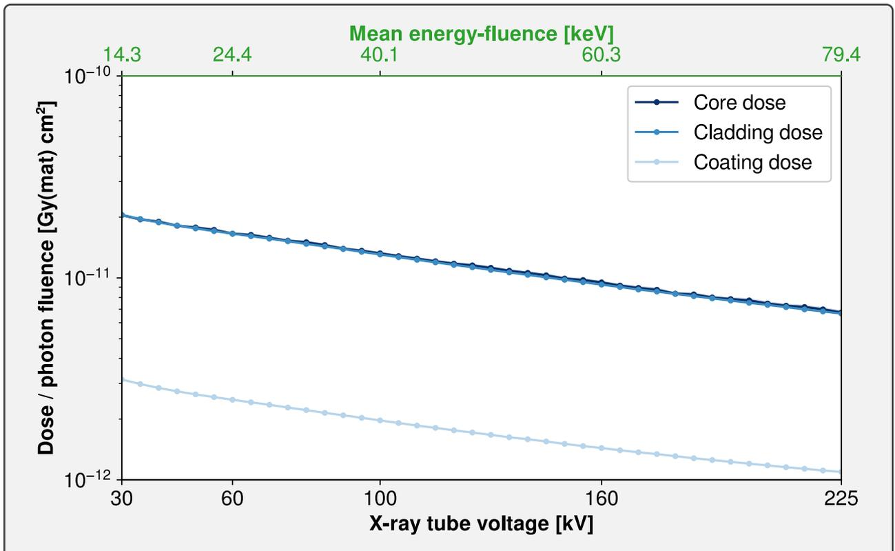
Figure 4.12. – Geant4 simulated dose/fluence of the different components of fiber **A** irradiated under X-rays with different tube voltages. Corresponding mean energy-fluences are given for reference.
