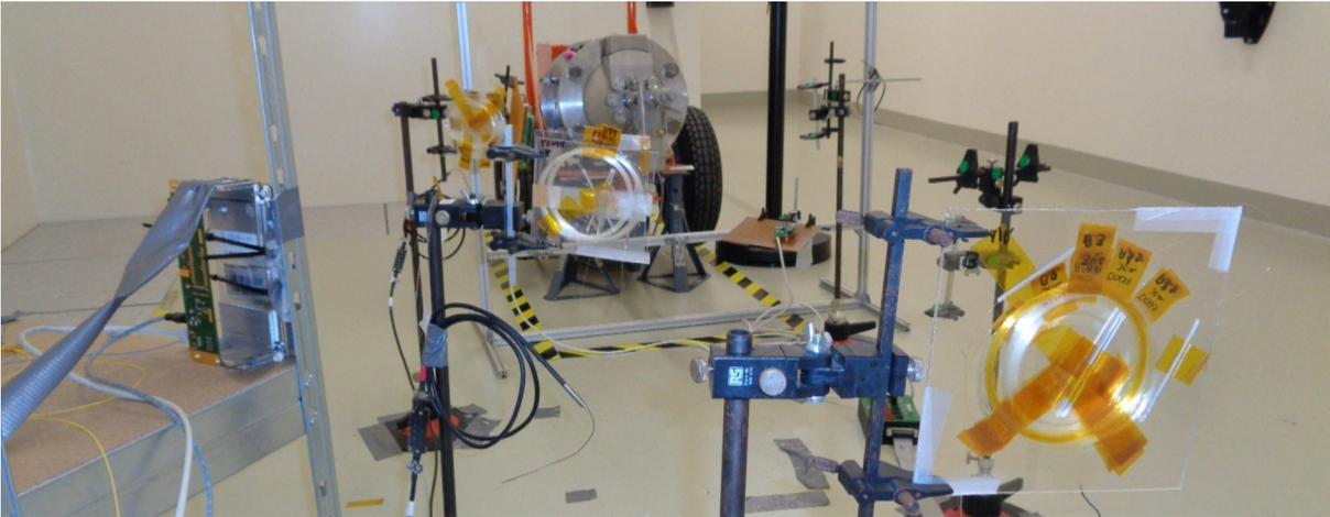
**Figure 3.18.** – Photograph of the Micro iOTDR  $\gamma$  ray irradiation setup. The irradiated Micro iOTDR device is on the left, and several optical fiber samples installed on transparent vertical supports can be seen at different distances from the source in the middle.
