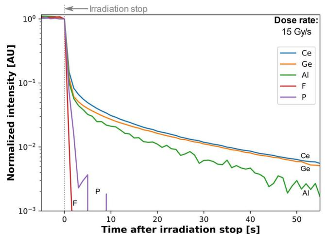
Fig. 6. Comparison of RL afterglow at 15 Gy/s of all tested fiber samples, normalized by the intensity measured at the end of irradiation. Values lesser than  $10^3$  were clipped for clarity.
