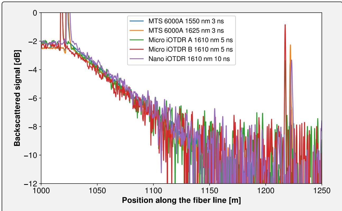
Figure 3.3. – Sample data of a region of interest (attenuating fiber). Device name, wavelength and pulse width are shown in the legend, with a common scan time of 10 s.
