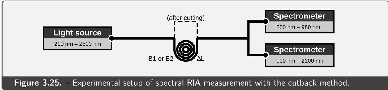
Figure 3.25. – Experimental setup of spectral RIA measurement with the cutback method.
