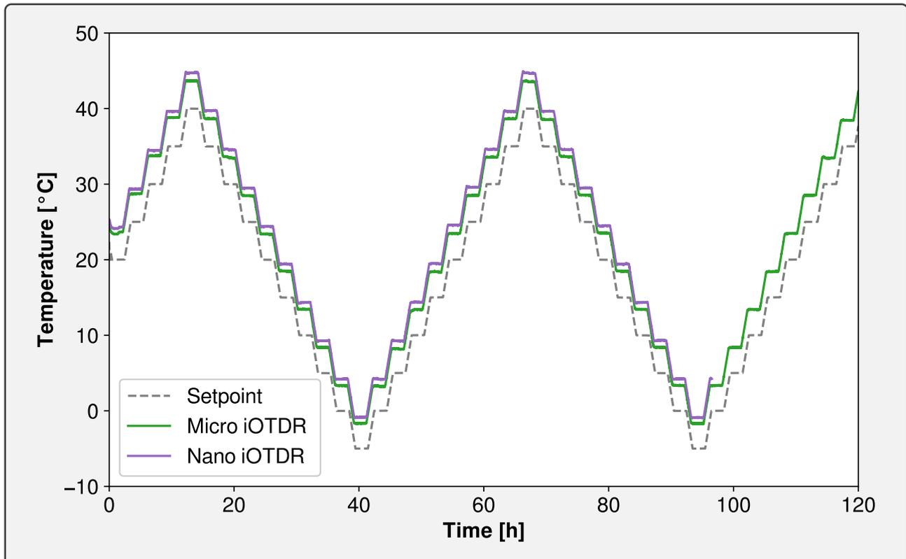
**Figure 3.13.** – Evolution of the heating/cooling chamber temperature setpoint (in dashed line), along with the temperature measured by thermocouples on the surface of the iOTDR devices (in solid lines), for the duration of the experiment.
