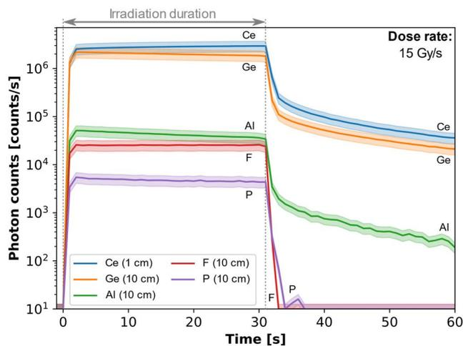
Fig. 5. Comparison of RL response of all tested fiber samples as a function of time, at the maximum dose rate of 15 Gy/s. Values lesser than  $10^1$  were clipped for clarity. Filled areas show the uncertainty range of  $\pm 25\%$ .
