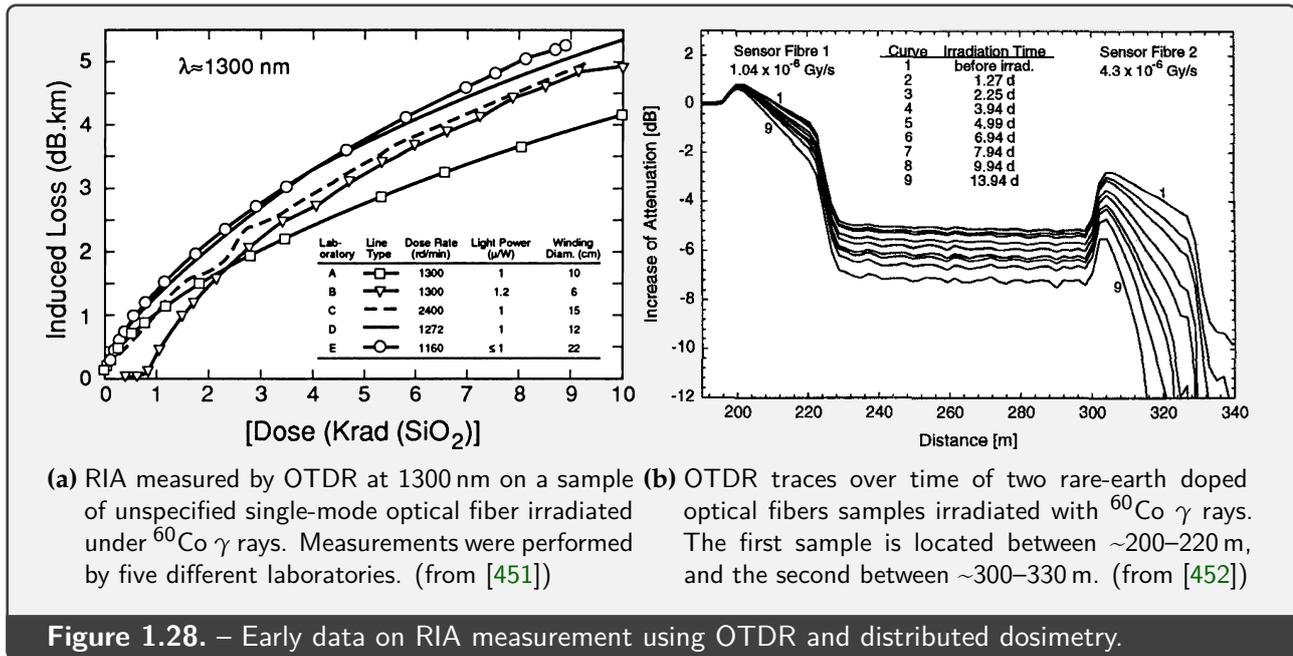
Figure 1.28. – Early data on RIA measurement using OTDR and distributed dosimetry.
