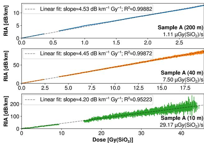
Fig. 3. Evolution of RIA (at 1610 nm) of sample A according to dose at different  $\gamma$  rays dose rates, during the first month of irradiation. A linear fit is applied on each curve (dashed lines) to visually highlight the linearity of these measurements.
