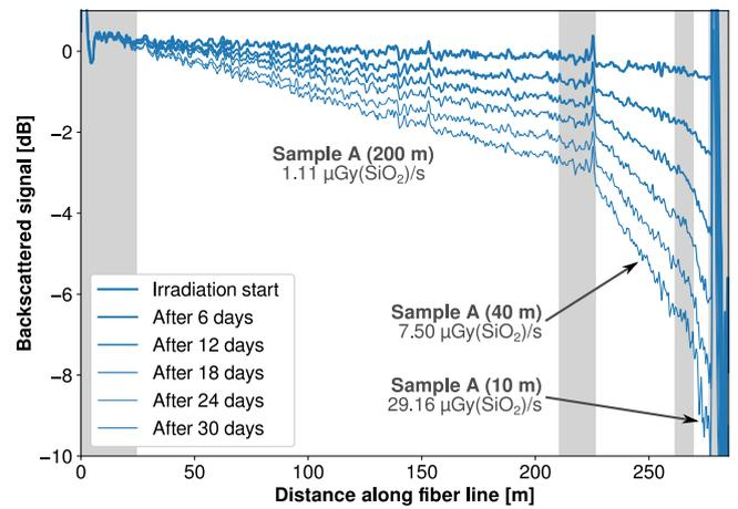
Fig. 2. OTDR traces (1610 nm) of measurement line A irradiated under  $\gamma$  rays during the first month of irradiation. Areas shown on a white background are the ones taken into account for RIA calculation.
