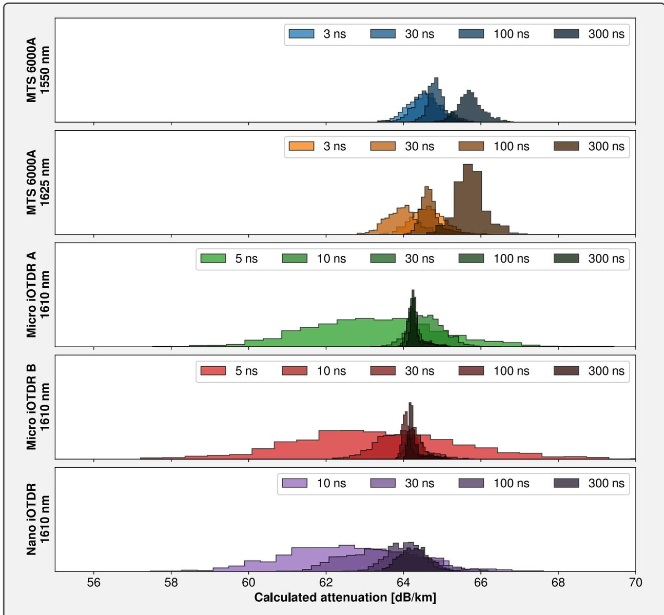
Figure 3.10. – Histograms of calculated attenuation values of the attenuating fiber segment over ~1200 measurements for all investigated devices and pulse widths, using a scan time of 10 s.
