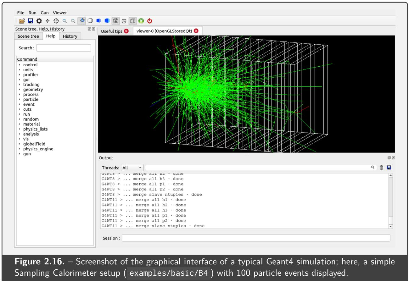
**Figure 2.16.** – Screenshot of the graphical interface of a typical Geant4 simulation; here, a simple Sampling Calorimeter setup ( examples/basic/B4 ) with 100 particle events displayed.
