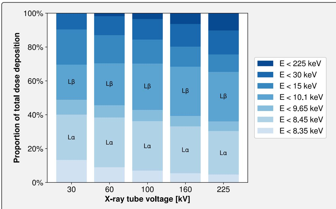
**Figure 4.15.** – Stacked bar plot of the simulated cumulative dose response in the core of fiber **A** irradiated under X-rays with different tube voltages. Contributions due only to tungsten characteristic X-ray lines  $L\alpha$  and  $L\beta$  are also annotated.
