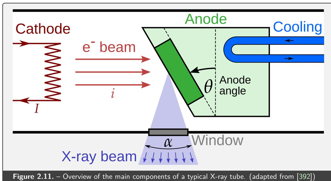
**Figure 2.11.** – Overview of the main components of a typical X-ray tube. (adapted from [392])
