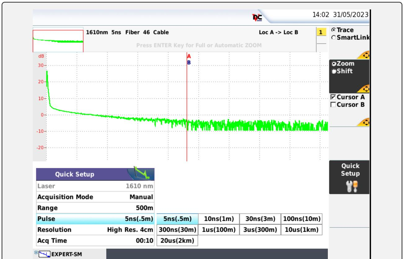
**Figure 2.6.** – Screenshot of the main parameter setting screen of a Micro iOTDR device. The highlighted choice is pulse width, and the list displayed to the right shows the available pulse widths selectable on this device, from 5 ns to 20  $\mu$ s. The lengths indicated in parentheses are the theoretical spatial resolutions linked to each pulse width.
