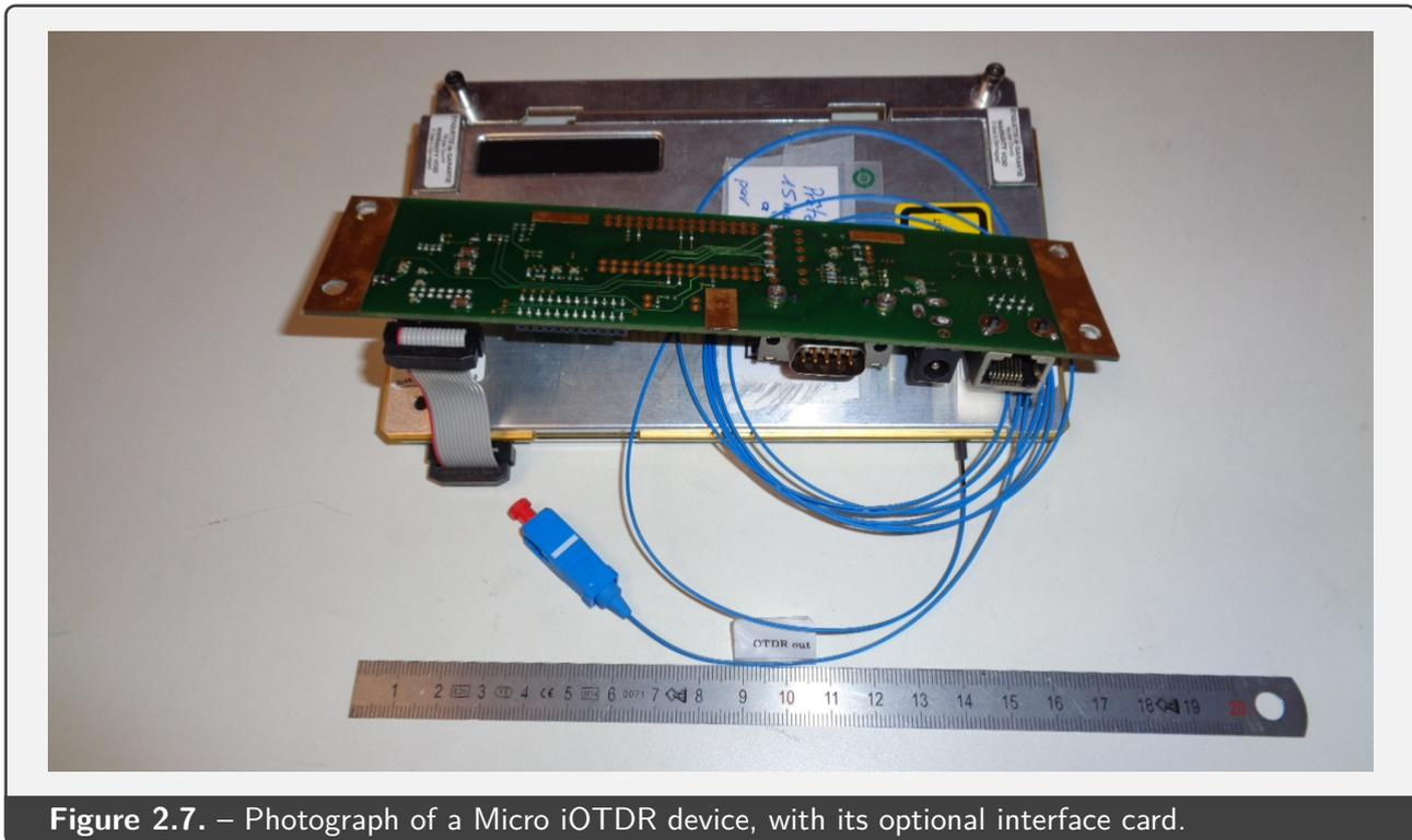
**Figure 2.7.** – Photograph of a Micro iOTDR device, with its optional interface card.
