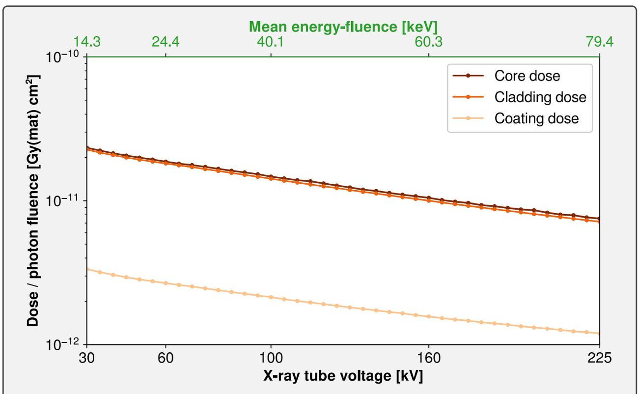
Figure 4.13. – Geant4 simulated dose/fluence of the different components of fiber **B** irradiated under X-rays with different tube voltages. Corresponding mean energy-fluences are given for reference.
