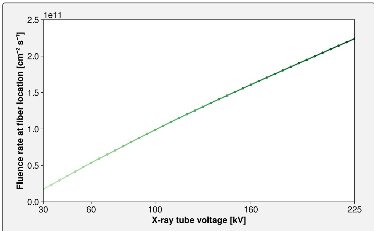
**Figure 4.11.** – SpekPy simulated fluence rate of X-rays irradiating an optical fiber coil placed around the beam maximum at a position  $y = 0$  and  $z = 42.5$  cm, for all investigated voltages.
