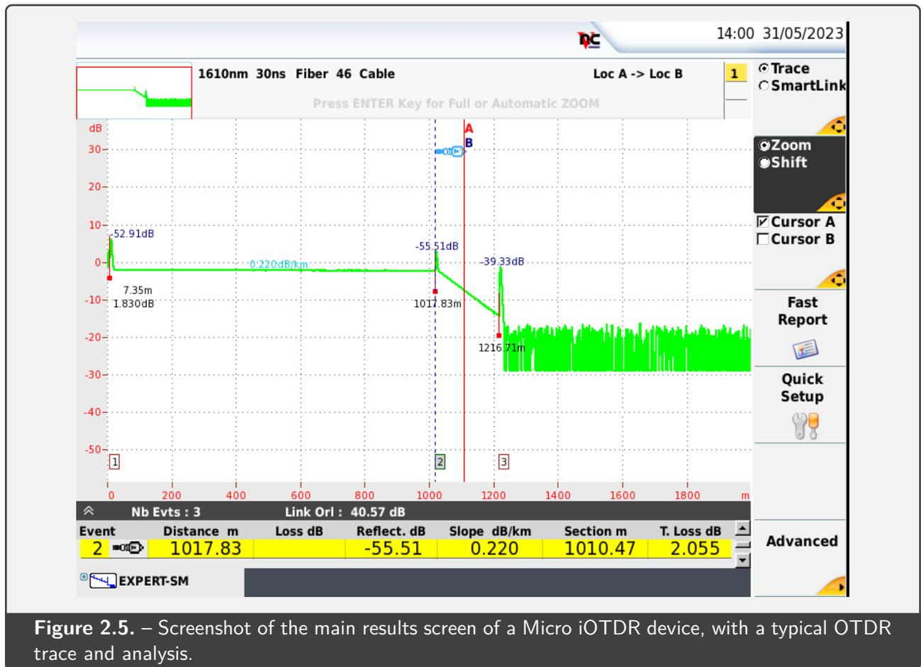
**Figure 2.5.** – Screenshot of the main results screen of a Micro iOTDR device, with a typical OTDR trace and analysis.
