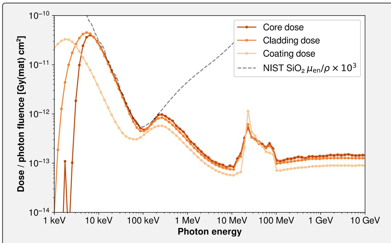
**Figure 4.3.** – Geant4 simulated dose/fluence of the different components of fiber **B** irradiated with photons. The mass-energy absorption coefficient for silica is plotted in dashed line, for comparison.
