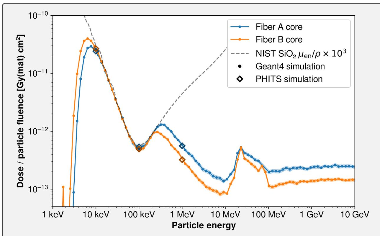
**Figure 4.4.** – Comparison of dose deposited by photons in the cores of fibers **A** and **B**. The mass-energy absorption coefficient for silica is plotted in dashed line. Geant4 data are indicated by dots, and PHITS data by diamonds.
