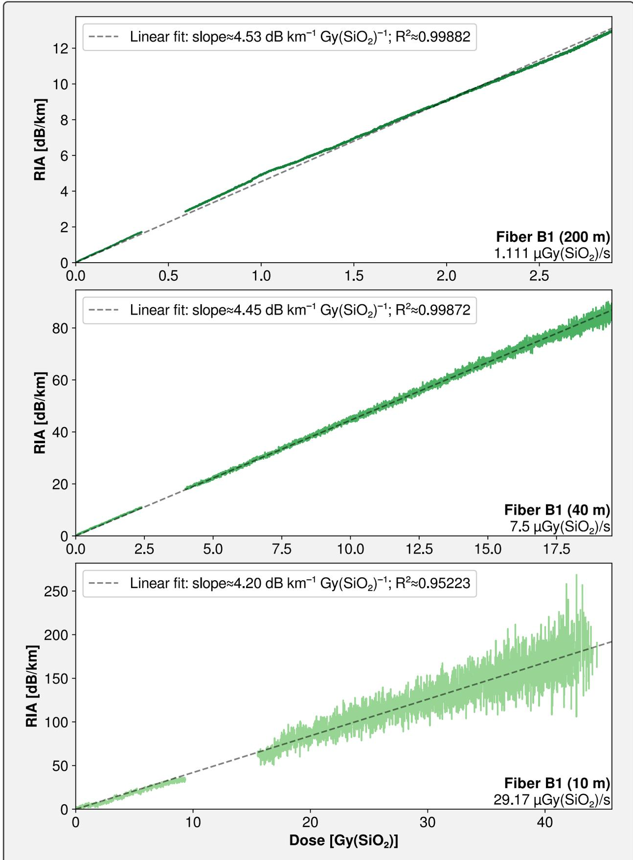
**Figure 3.20.** – RIA at 1610 nm as a function of dose for each segment on the measurement line connected to Micro iOTDR A, during the first month of irradiation. Linear fit of each of these data sets is shown in dashed line.
