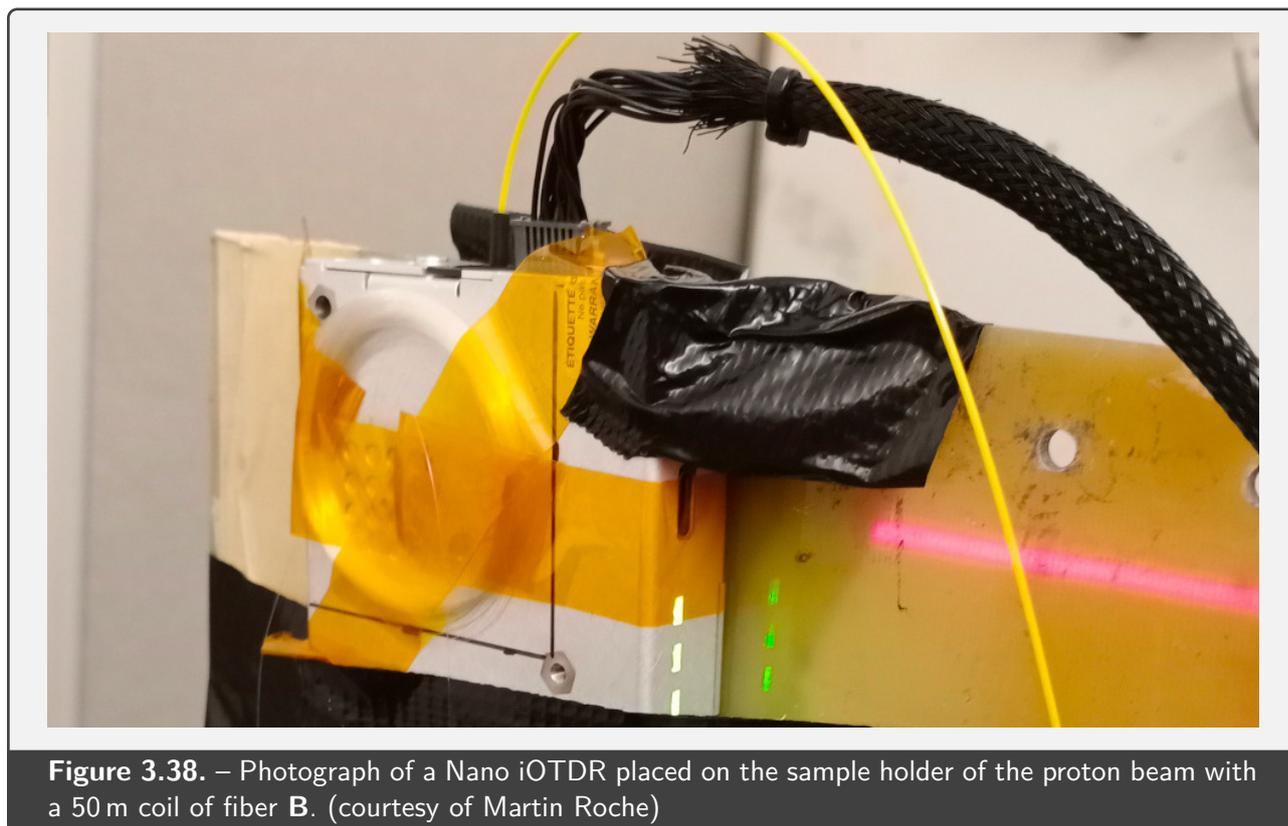
**Figure 3.38.** – Photograph of a Nano iOTDR placed on the sample holder of the proton beam with a 50 m coil of fiber B. (courtesy of Martin Roche)
