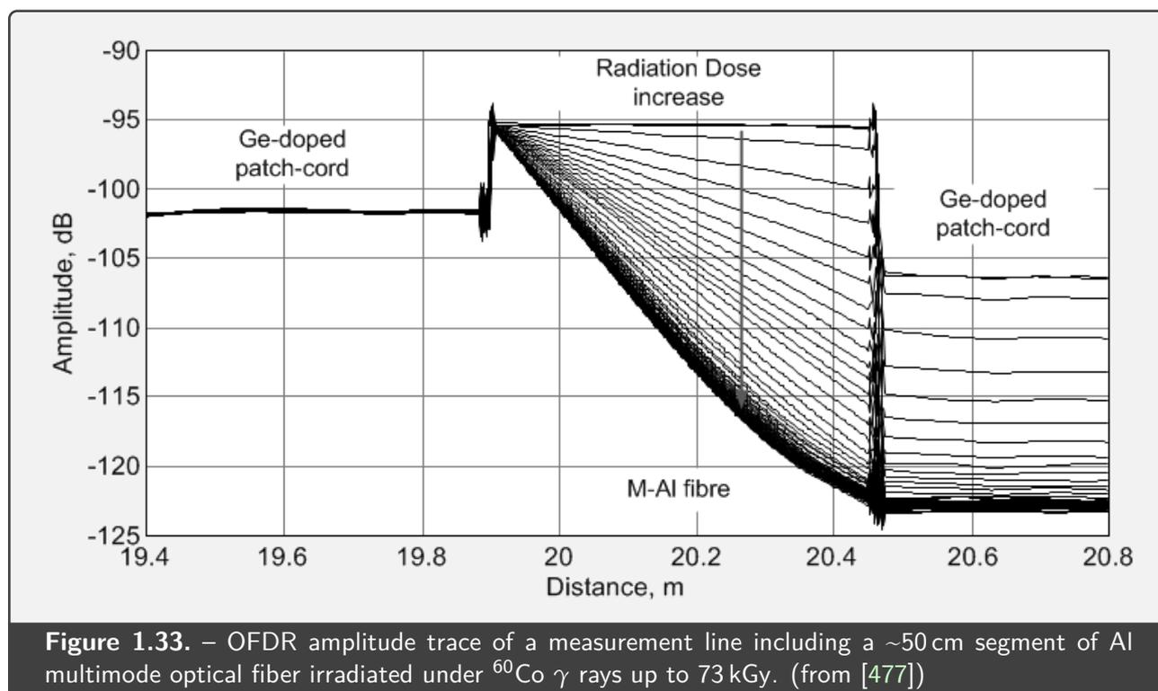
**Figure 1.33.** – OFDR amplitude trace of a measurement line including a ~50 cm segment of Al multimode optical fiber irradiated under  $^{60}\text{Co}$   $\gamma$  rays up to 73 kGy. (from [477])
