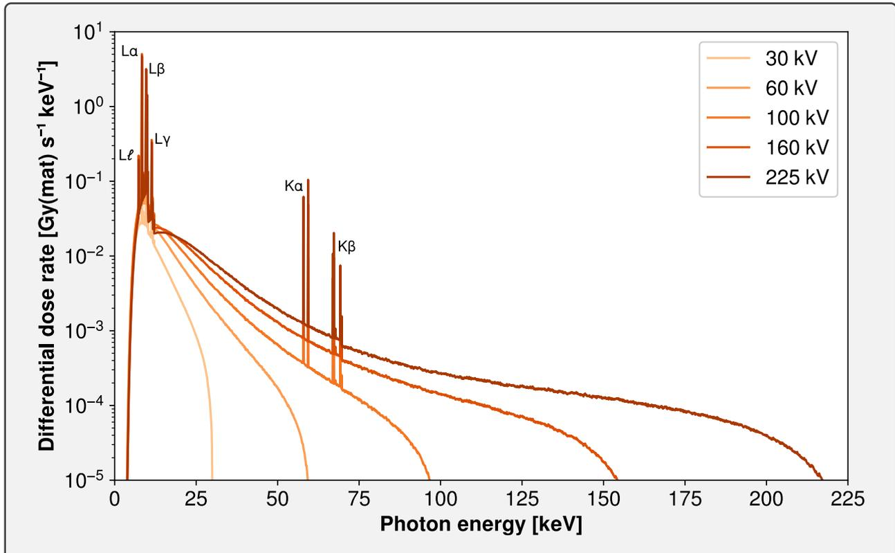
Figure 4.16. – Simulated differential dose response spectrum of in the core fiber **B** irradiated under X-ray with different tube voltages. The main tungsten characteristic X-ray lines are also annotated.
