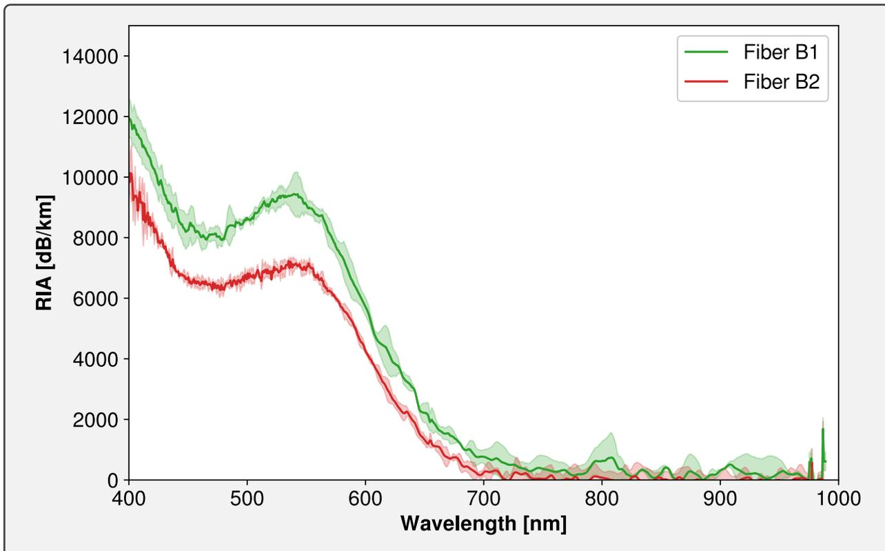
**Figure 3.26.** – Spectral RIA, in the visible domain, of the **B1** and **B2** samples irradiated under  $\gamma$  rays at a dose of 12.9 Gy(SiO<sub>2</sub>). Filled areas in lighter color show uncertainties at  $\pm 2\sigma$ .
