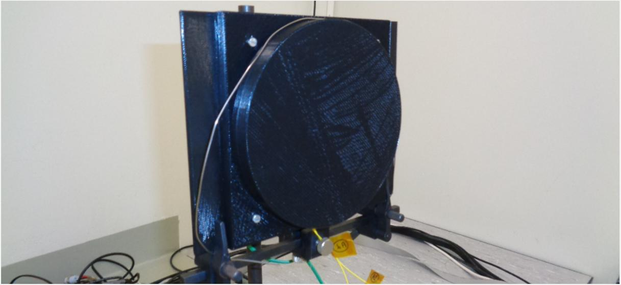
**Figure 3.29.** – Photograph of the cover box used to isolate optical fibers from ambient lighting in the  $\gamma$  ray irradiation experiment involving Nano iOTDR.
