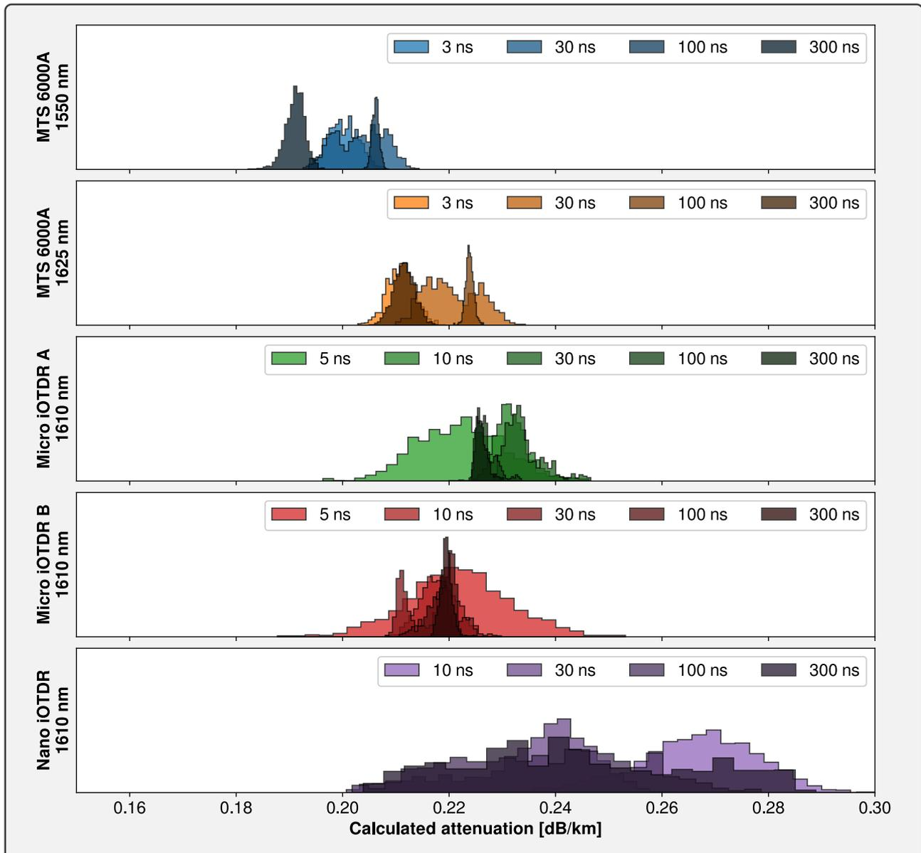
Figure 3.8. – Histograms of calculated attenuation values of the launch fiber segment over ~1200 measurements for all investigated devices and pulse widths, using a scan time of 10 s.
