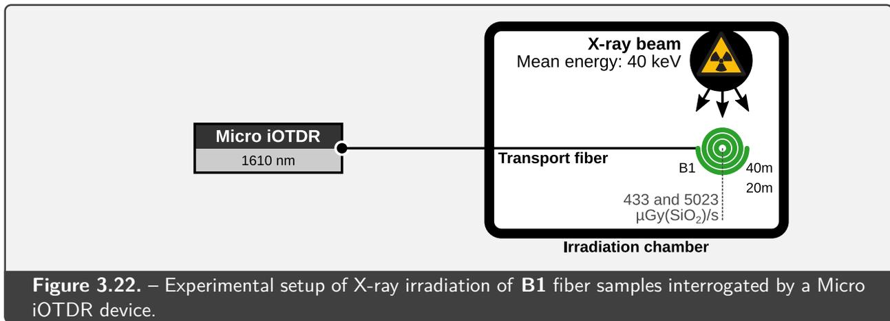
**Figure 3.22.** – Experimental setup of X-ray irradiation of B1 fiber samples interrogated by a Micro iOTDR device.
