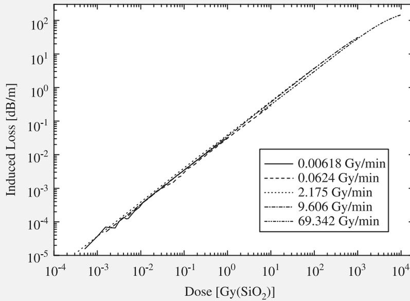
**Figure 1.29.** – Calibration curve under  $^{60}\text{Co}$   $\gamma$  rays of the Ge-P co-doped fiber selected for distributed dosimetry of the TTF1 facility in DESY Hamburg. Measurements were performed at room temperature with  $\lambda = 678$  nm at five dose rates, indicated by different line styles. (from [398])
