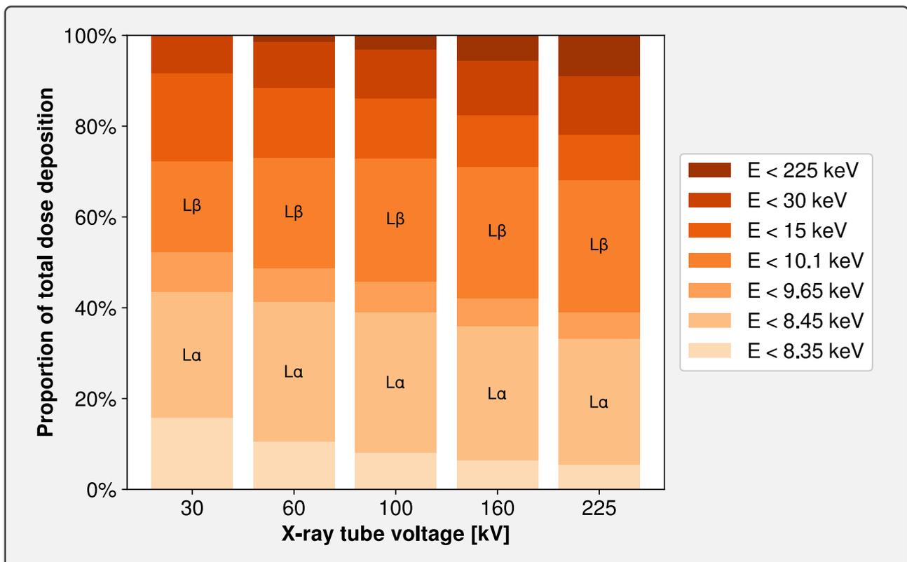
Figure 4.17. – Stacked bar plot of the simulated cumulative dose response in the core of fiber **B** irradiated under X-rays with different tube voltages. Contributions due only to tungsten characteristic X-ray lines  $L\alpha$  and  $L\beta$  are also annotated.
