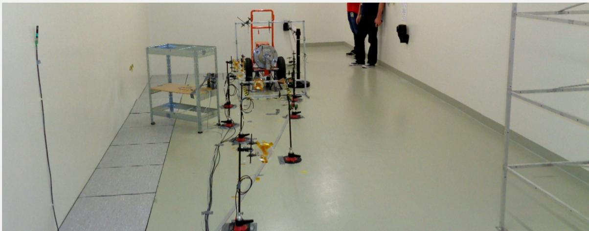
**Figure 2.13.** – Photograph of the PRESERVE  $\gamma$  ray irradiation facility in 2021. The  $^{60}\text{Co}$  source is installed at the center of the picture, on the orange structure.
