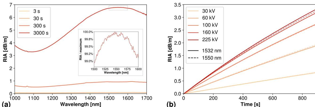
**Figure 8.** (a) Spectral RIA of the optical fiber irradiated during 3, 30, 300 and 3000 s with a tube voltage of 100 kV. Inset magnifies the framed area at 3000 s between 1500 nm and 1600 nm, normalized by maximum. (b) Evolution of optical fiber RIA at 1532 nm and 1550 nm according to irradiation time, at different X-ray tube voltages.
