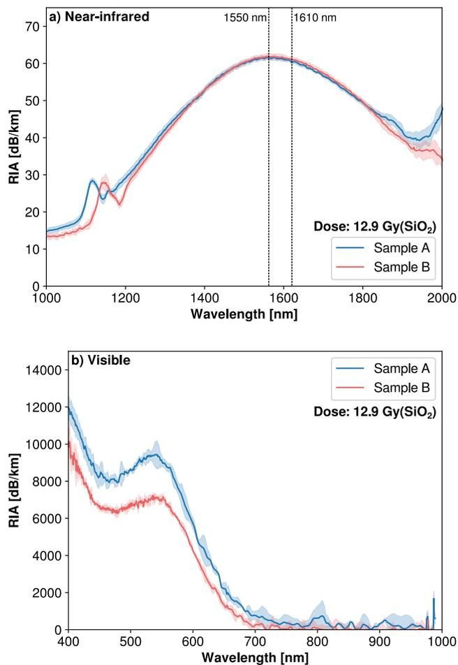
Fig. 7. RIA spectra in (a) near-infrared domain and (b) visible domain of OF samples A and B irradiated under  $\gamma$  rays at a dose of 12.9 Gy(SiO<sub>2</sub>). Filled areas in lighter color show uncertainties at  $\pm 2\sigma$ .
