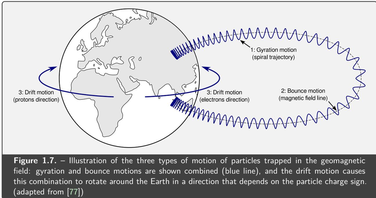
**Figure 1.7.** – Illustration of the three types of motion of particles trapped in the geomagnetic field: gyration and bounce motions are shown combined (blue line), and the drift motion causes this combination to rotate around the Earth in a direction that depends on the particle charge sign. (adapted from [77])
