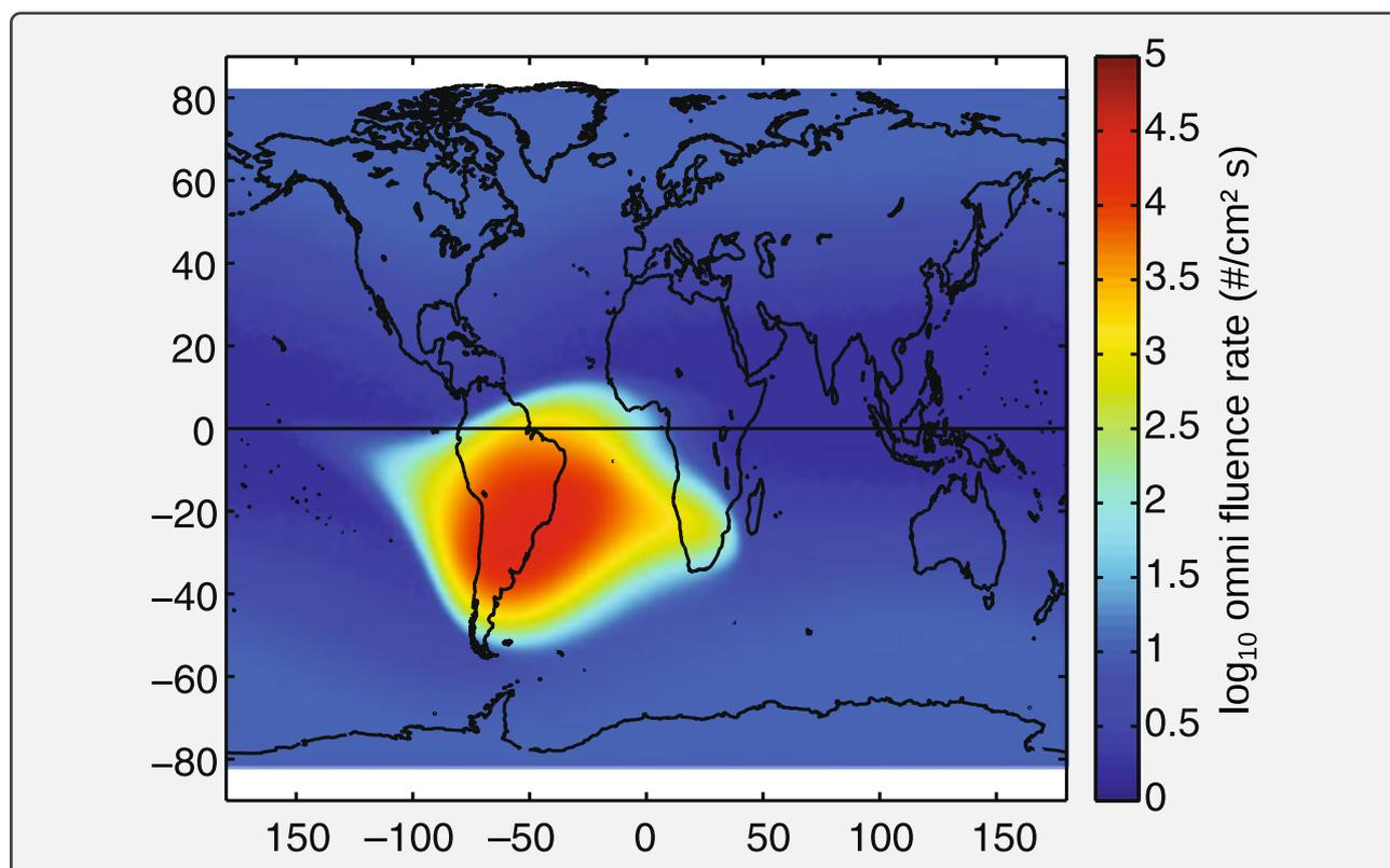
**Figure 1.10.** – Mapping of the median  $> 36$  MeV proton omnidirectional fluence rate measured over 13 years by the satellite POES N15, at an altitude of  $\sim 840$  km. The outstanding area of high intensity located above South America is the *South Atlantic Anomaly* (SAA). (adapted from [102])
