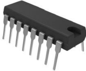
Figure 2.4 DIP: Dual in-line [12]
