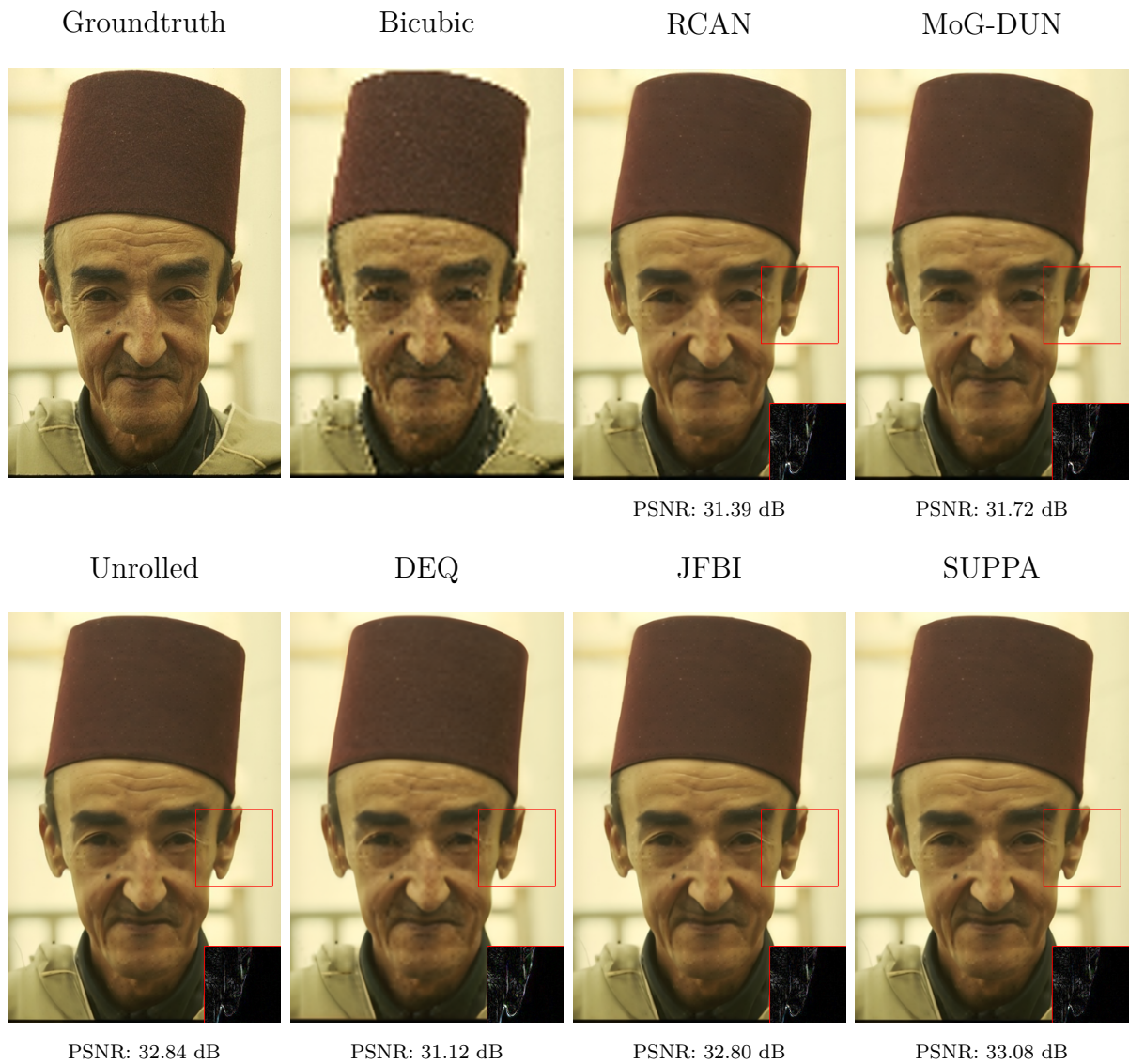
Figure 2.4 – Visual comparisons of image super-resolution of different methods with a bicubic downsampling (x4) without anti-aliasing and with a bicubic interpolation initialization on a sample image from the BSDS100 dataset [101]. A portion of the error map is selected to highlight the error in a specific area. The error is amplified by a factor of 3.
